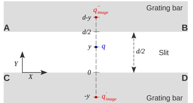
FIG. 2. A cross-sectional view of the diffraction grating. ABCD is one of the slit openings in the grating. AB and CD are the planes of two neighboring bars of the grating. Since the grating is made of metal, image charges ( $q'_{image}$  and  $q''_{image}$ ) are induced due to a charge  $q$  situated at a distance  $y$  from the lower plane (CD). The width of the slit is  $d/2$ .
