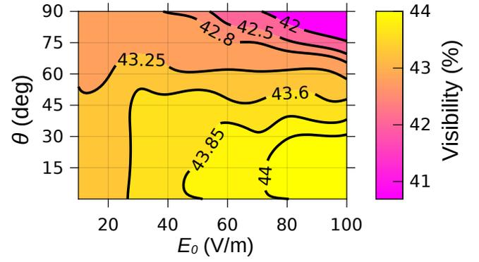
FIG. 10. Variation of the fringe visibility ( $V$ ) as a function of magnitude  $E_0$  and orientation ( $\theta$ ) of the applied uniform electric field.
