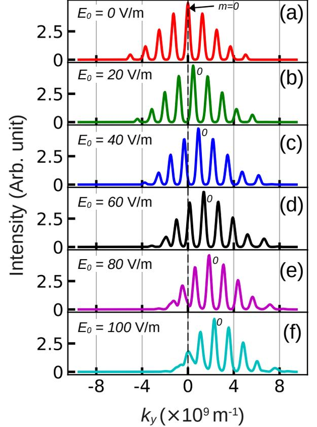
FIG. 7. Fringe pattern in the momentum space ( $k_x, k_y$ ) for different magnitudes of electric fields (a)  $E_0 = 0$  V/m, (b)  $E_0 = 20$  V/m, (c)  $E_0 = 40$  V/m, (d)  $E_0 = 60$  V/m, (e)  $E_0 = 80$  V/m, and (f)  $E_0 = 100$  V/m. The electric field is applied in the transverse direction ( $\theta = 90^\circ$ ).
