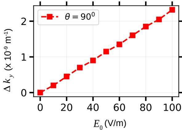
FIG. 5. Variation of the change in transverse wave number  $\Delta k_y$  of the diffracted wave packet with the applied uniform electric field strength  $E_0$ . The values of  $\Delta k_y$  are obtained at  $X_2 = 2L_T$  for the orientation of the electric field  $\theta = 90^\circ$ .
