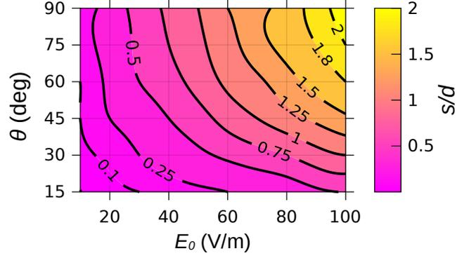
FIG. 8. Variation of fringe shift normalized by the grating period ( $s/d$ ) with the magnitude  $E_0$  and orientation ( $\theta$ ) of the applied uniform electric field.
