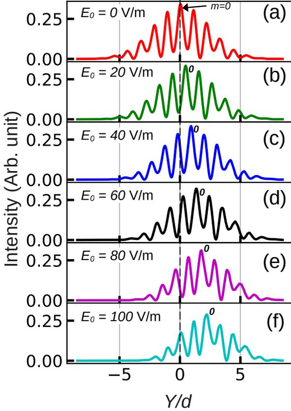
FIG. 6. Fringe pattern at  $X_2 = 2L_T$  for different magnitudes ( $E_0$ ) of the applied electric fields in the transverse direction ( $\theta = 90^\circ$ ). (a)  $E_0 = 0$  V/m, (b)  $E_0 = 20$  V/m, (c)  $E_0 = 40$  V/m, (d)  $E_0 = 60$  V/m, (e)  $E_0 = 80$  V/m, and (f)  $E_0 = 100$  V/m.
