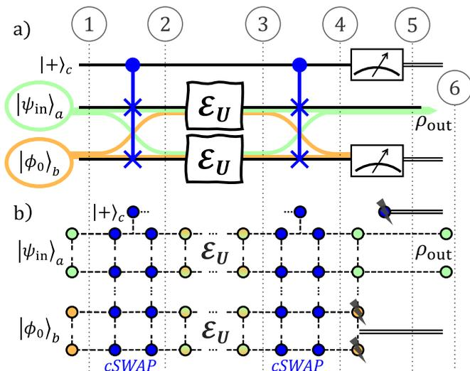
Figure 1. Illustration of the strategy for enhancing the fidelity of noisy gate-based (a) and measurement-based (b) computations. The protocol steps from one to six (described in the main text) are highlighted. The input (auxiliary) state follows the superposed green (orange) paths depending on the state of the control.
