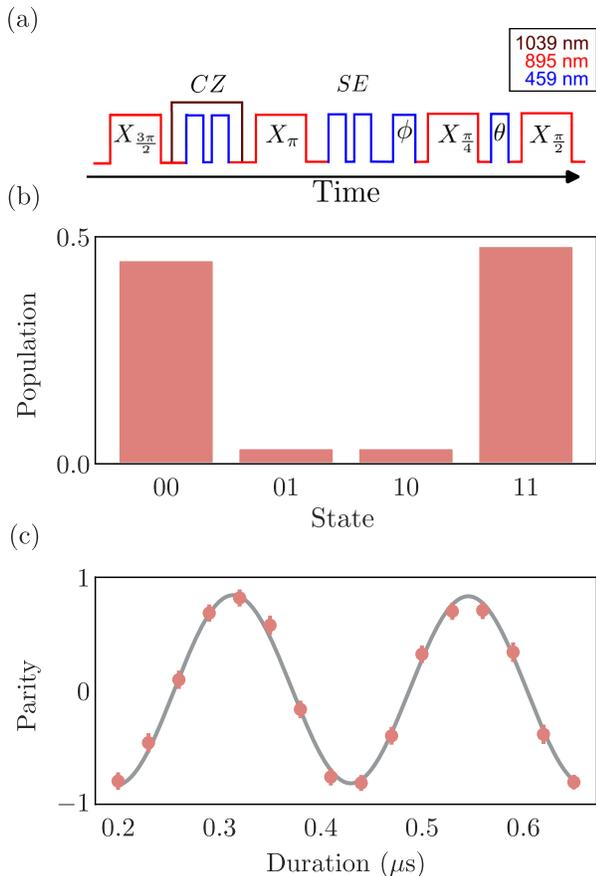
FIG. 5. (a) Pulse sequence used to create entangled Bell state  $|\Psi^+\rangle$  and analysis pulses for parity oscillation. (b) Output populations for a single pair giving  $P_{00} + P_{11} \geq 0.91(4)$ . (c) Parity oscillation with contrast  $C = 0.83(2)$ , giving a raw Bell state fidelity of  $F \geq 0.88(2)$ .
