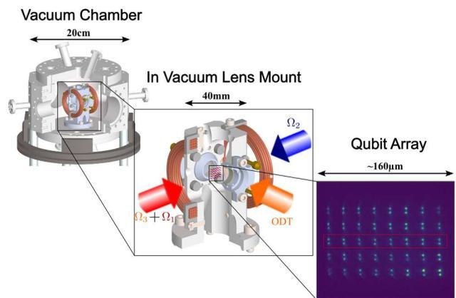
FIG. 1. Outline of our setup - a reconfigurable qubit array is created at the focus of in-vacuo lenses by a 1064 nm optical dipole trap (ODT). Global beams perpendicular to the dipole trap and along the quantisation axis enable qubit operations. Shown is an average image of 40 pairs of atoms. The work presented in this paper focuses on the central row highlighted by the red box to suppress variations coming from spatial uniformity of the Rydberg excitation lasers.
