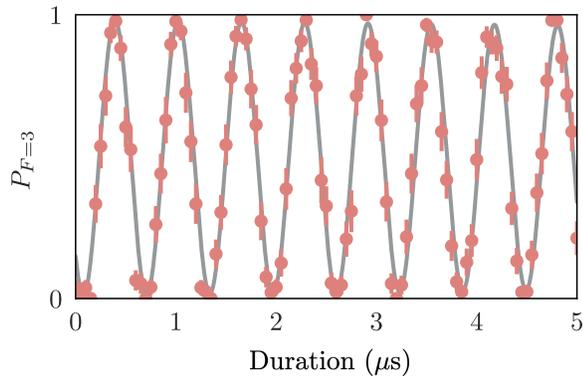
FIG. 3. Raman Rabi oscillation of a single site using our phase locked Raman system,  $\Omega_1/2\pi = 1.58(1)$  MHz at  $\Delta_1/2\pi = -250$  GHz. The standard deviation in Rabi frequency across our 16 sites is 0.5 %
