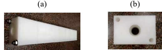
Fig. 2. 7 \times 10 \times 70 \text{ cm}^3 HDPE blocks with a 1-inch central hole where the neutron counters are embedded (a). The blocks consist of seven 7 \times 10 \times 10 \text{ cm}^3 smaller pieces (b) which are assembled using two stainless steel rods as shown in (a).
