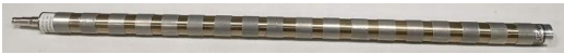
Fig. 1. 60-cm length and 1-inch diameter ^3\text{He} -filled proportional counter partially covered with cadmium to provide the detector with a flat efficiency.
