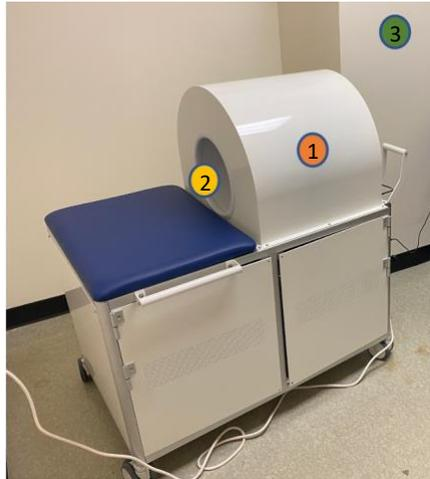
**Supplementary Figure 1.** The portable 0.05T scanner and the three locations used to measure temperature and humidity 1) inside the bore; 2) near the mouth of the bore; 3) in the room
