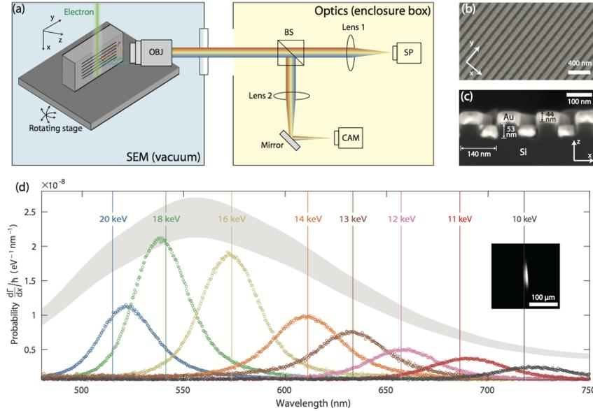
**Fig. 2** The bounds of Eq. (68) dictate upper limits to Smith–Purcell emission rates. (a–d) The experiments of Ref. [104] quantitatively confirm that designed metallic gratings can approach the fundamental performance limits. (Adapted from Ref. [104].)
