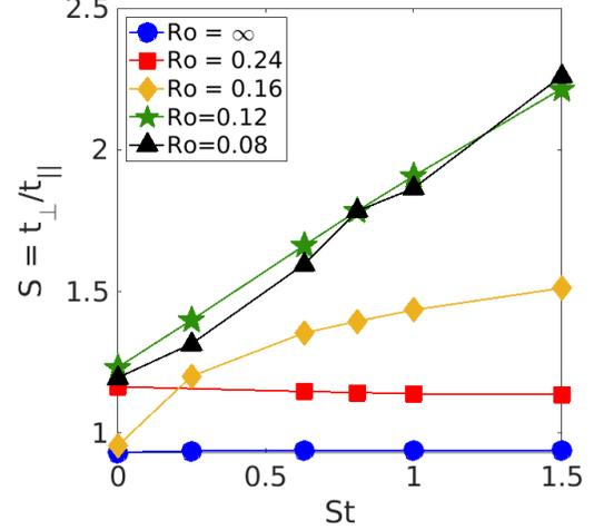
FIG. 8. Lagrangian anisotropy ratio  $S$  as a function of the Stokes number  $St$ , plotted for five different values to rotation rate (see legends).
