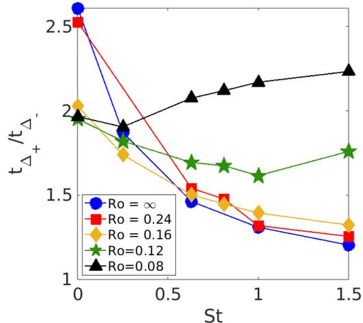
FIG. 6. Ratio of resident times of particles in vortical ( $t_{\Delta+}$ ) to that in straining ( $t_{\Delta-}$ ) as a function of Stokes numbers  $St$ . The curves are plotted for five different strengths of rotation  $Ro = \infty, 0.24, 0.16, 0.12,$  and  $0.08$  as marked by the legends.
