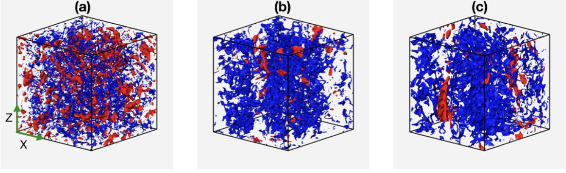
FIG. 2. Volume visualization of isosurfaces of vorticity magnitude ( $|\omega| = |\nabla \times \mathbf{v}|$ ) for three different values of rotation rates (a)  $Ro = \infty$ , (b)  $Ro = 0.16$ , and (c)  $Ro = 0.08$ . The blue and red colored isosurfaces represent weak ( $|\omega| = 0.5$ ) and intense vorticity ( $|\omega| = 7$ ) magnitudes, respectively.
