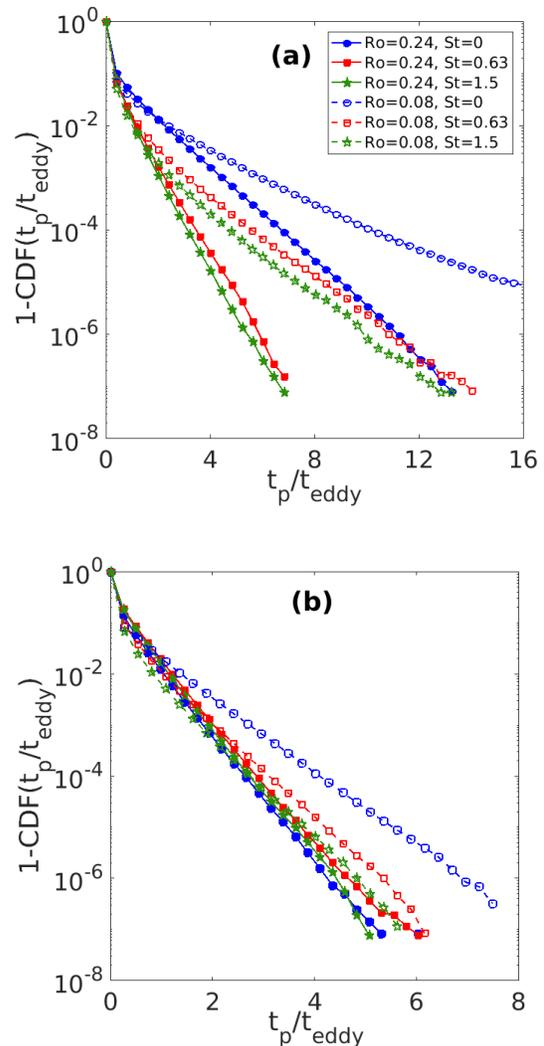
FIG. 5. Cumulative distribution functions (CDFs) of persistence time  $t_p$  of particles in (a) vortical ( $\Delta \geq 0$ ) and (b) straining ( $\Delta < 0$ ) regions. The CDFs are plotted for two different strengths of rotation ( $Ro = 0.24$  and  $0.08$ ) and three different values of Stokes number ( $St = 0, 0.63$ , and  $1.5$ ) as shown by the legends.
