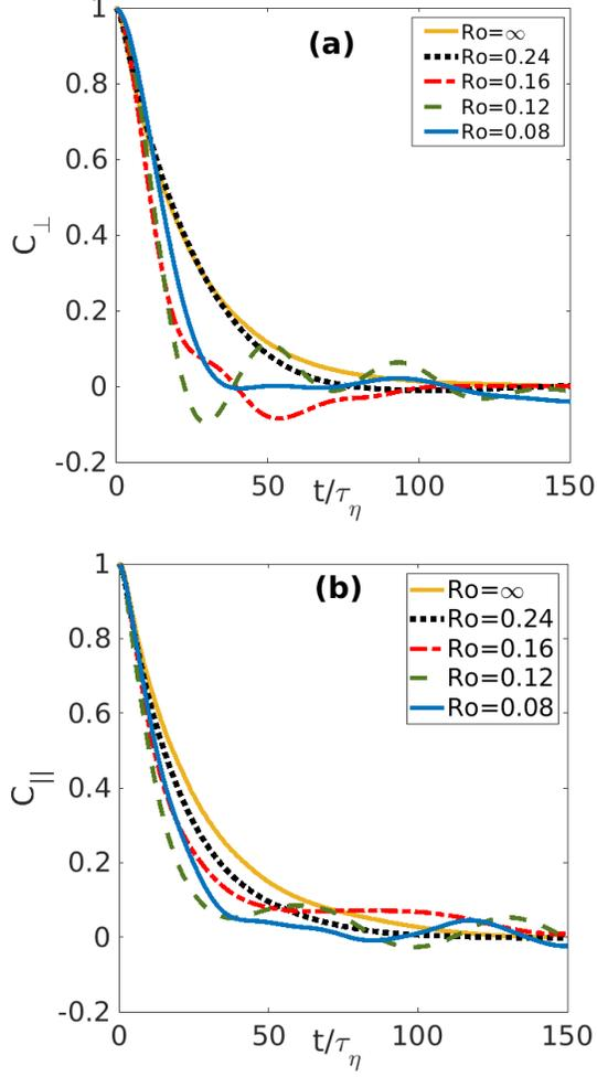
FIG. 7. Autocorrelations of Lagrangian velocities of tracers in the plane (a) perpendicular and (b) parallel to the axis of rotation as a function of time. The plots are for five different values of rotation rates  $Ro = \infty, 0.24, 0.16, 0.12, \text{ and } 0.08$ .
