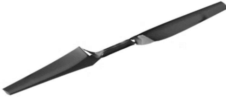
**Fig. 2.** Shape model of the NREL Phase VI wind turbine blade.
