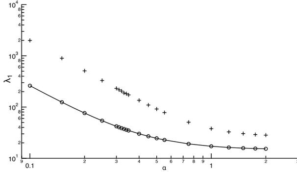
Figure 5. Variation of the smallest eigenvalue  $\lambda_1$  with respect to  $\alpha$ . Solid line is analytical eigenvalue (2). Circle and cross indicate eigenvalues for the cases of “ $u_r = 0$ ” and “ $u_\theta = 0$ ”, respectively. The eigenvalue of the  $u_r$ -free mode, less than that of the  $u_\theta$ -free mode, agrees with that of the standard mode, Eq. (2), and the corresponding distribution, omitted due to space constraints, also agrees with that of the standard mode (3).
