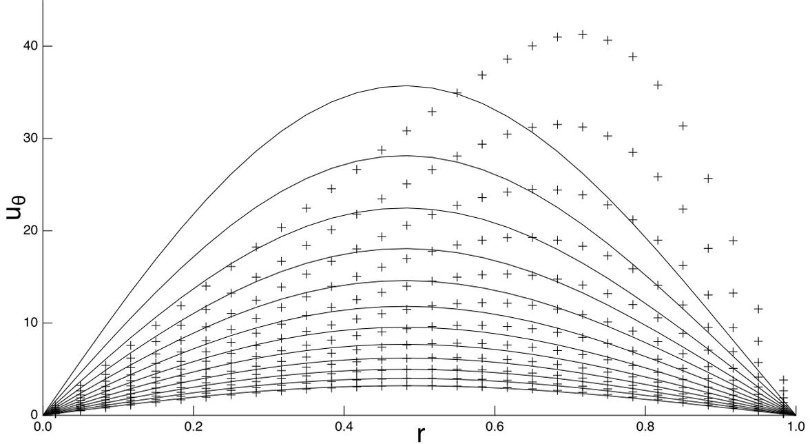
Figure 7. Decays of the distribution of azimuthal velocity component from  $t = 0.05$  to  $0.16$  ( $N = 30$ ). The distribution and its corresponding correlation Bessel function are indicated by plus marker and solid line, respectively. The uppermost is at  $t = 0.05$ , and time increments are  $0.01$ . The lowermost distribution agrees well with the Bessel function: the correlation coefficient exceeds  $0.995$  at  $t = 0.16$ .
