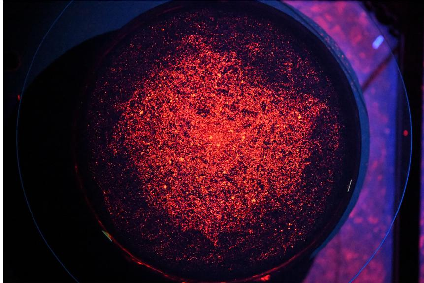
Figure 2. An example of a photo of a fluorescent top surface, illuminated by an ultraviolet torch.
