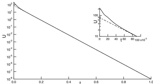
Figure 6. Variation of top-surface-mean speed with respect to time  $t$ . The magnification is at around  $t = 0$ . Dotted and solid lines indicate the variations for  $N = 20$  and  $30$ , respectively. But they are overlapped. For  $t > 0.059$  the solid line agrees well with its exponential correlation function, indicated by dashed line, and recovers the decay rate of  $22.788(=\lambda_{SDM})$  with the relative error of  $0.0092\%$ .
