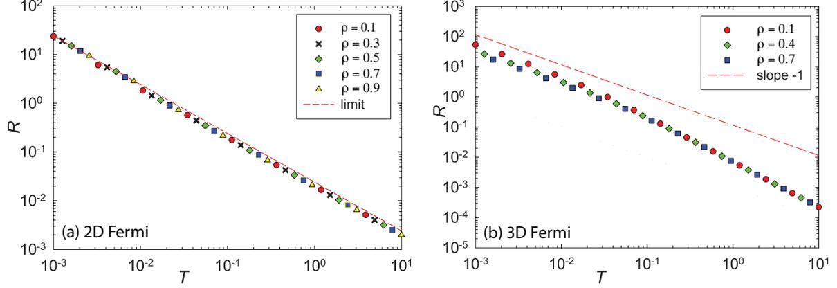
Figure 1:  $R$  versus  $T$  for the two and three-dimensional ideal Fermi gases, each for several constant values of  $\rho$ . (a) For small  $T$ , the 2D case has all the points fall on the same curve, with limiting slope  $-1$ . (b) For small  $T$ , the 3D case shows a density dependence, but for each density the limiting points all fall on a curve with slope  $-1$ .
