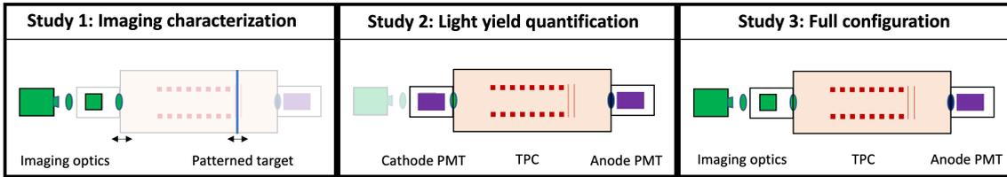
**Figure 1:** The three system configurations in which experimental data reported in this paper were collected.
