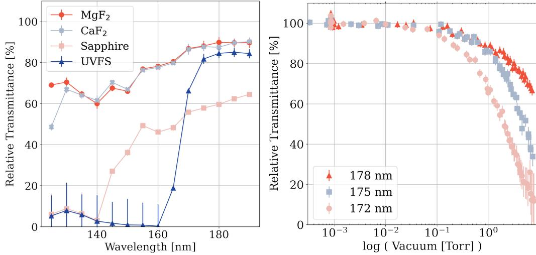
**Figure 7:** Measurement of relative transmittance for 5 mm-thick windows of various materials (Left) and vacuum levels (Right), as measured with a deuterium lamp and diffraction grating to select wavelength. Uncertainties in measurements are statistical only.
