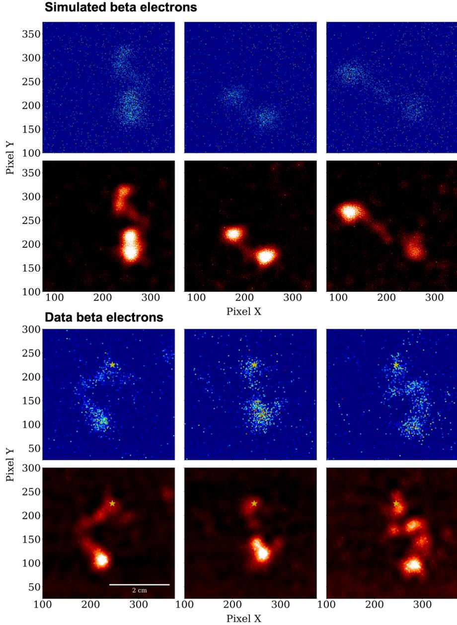
**Figure 16:** Simulated (Top) and detected (Bottom) beta electrons in NEXT-CRAB-0. The blue images are before filtering and the red images are after the filtering protocol is applied.
