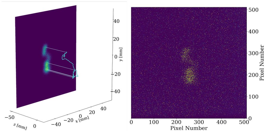
**Figure 9:** One simulated camera captured event track, consisting of two beta decays. Left: Simulated 2D electron distribution. Right: A simulated camera image of the same event, generated via the techniques in Section 3.2.
