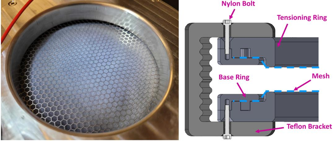
**Figure 3:** Left: Picture of mesh tensioned within its frame. The frame that holds the mesh is also used to do the tensioning. Right: Section view of the EL region. As the two frames are bolted together, the lip of the top ring presses down on the mesh and stretches it past the base ring as shown by the blue dashed line. The nylon bolts replace some of the metal-tensioning screws to hold the rings in place on the Teflon brackets.
