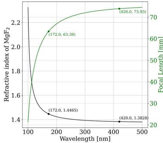
**Figure 6:** Refractive index and focal length of a 28.3 mm radius of curvature  $\text{MgF}_2$  lens vs wavelength.
