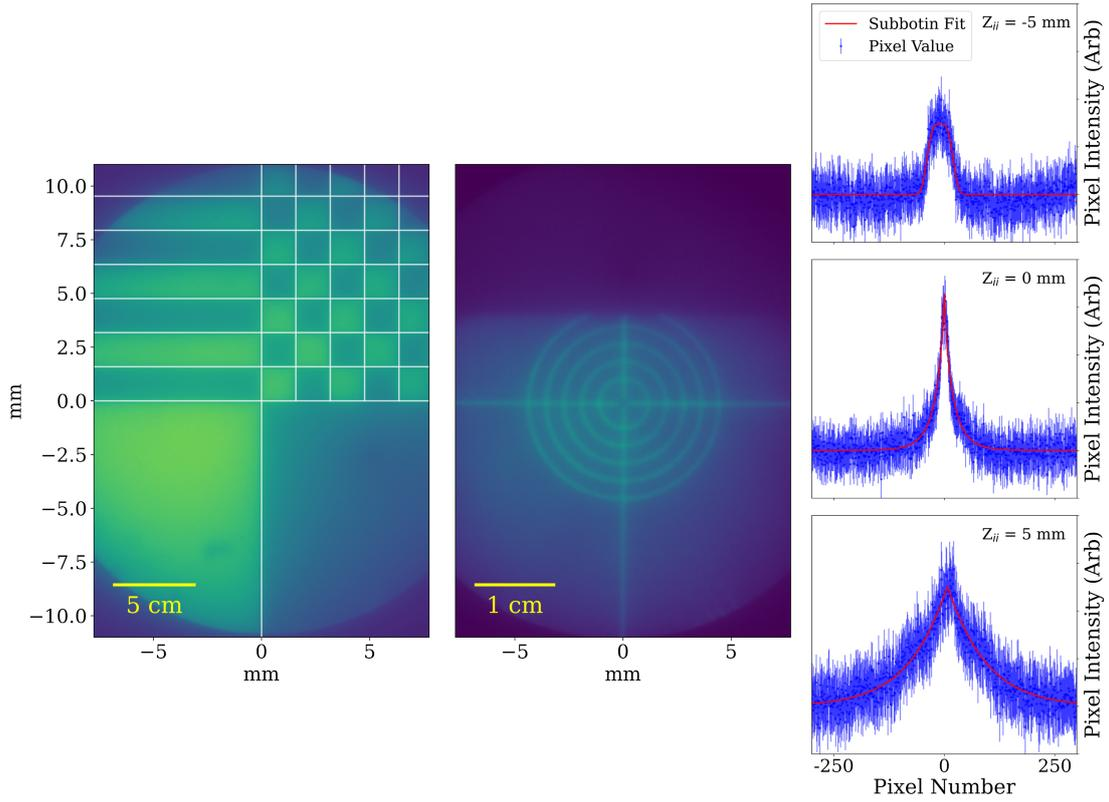
**Figure 12:** Left and center: Image of the *ex-situ* targets as imaged by the FLIR Firefly camera and the image intensifier. Right: The averaged profile of the target line with the image intensifier at varying on-axis locations. The red line shows the function fit to these values using Eq. 4.1. This process was repeated at each recorded position in Fig. 13 for both moving optical components.
