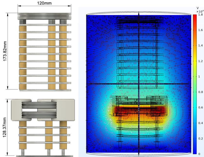
**Figure 4:** Left: A schematic of the inner elements of the TPC. Right: An electric potential simulation of the inside of the chamber using COMSOL. The colors in the COMSOL simulation represent the electrical potentials applied while the lines represent the electric field, with the arrows pointing in the field line directions.
