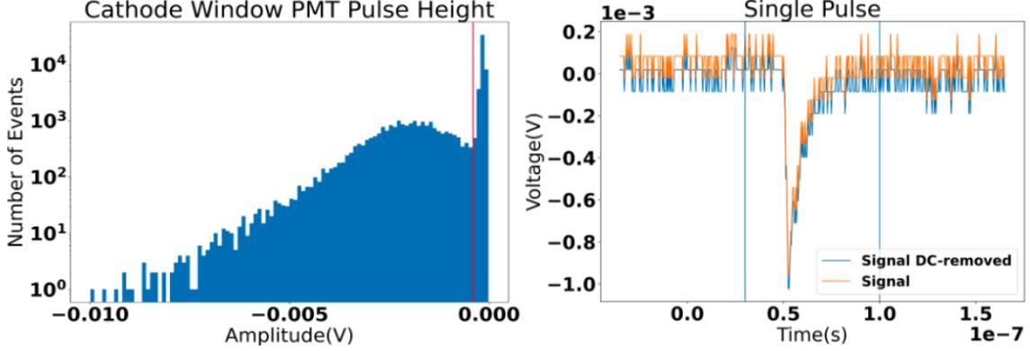
**Figure 20:** Left: Pulse height spectrum for the cathode window PMT. The red line indicates a rough cut made to separate the SPE peak from noise. Right: Example SPE waveform used in the calibration procedure, before and after baseline subtraction.
