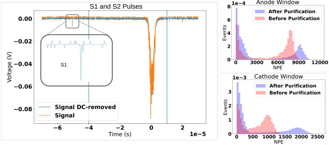
**Figure 14:** Left: Example of a single triggered data event showing S1 and S2 pulses. The raw signal (orange) is corrected by a DC offset factor to get the DC-removed signal (blue). The two blue lines represent the integration window of the S2 signal. Right: total detected light yield distributions at each PMT, before and after gas purification.
