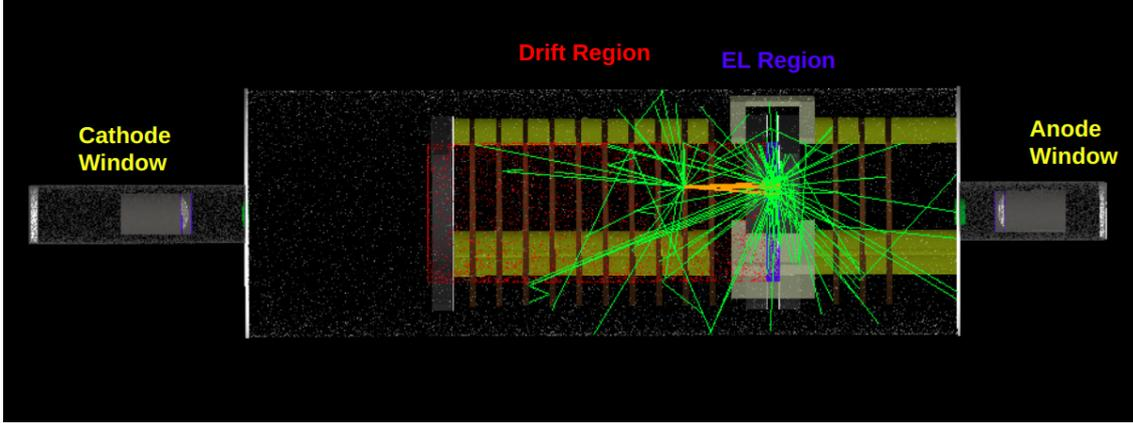
**Figure 8:** The NEXT-CRAB-0 detector geometry rendered in GEANT4.
