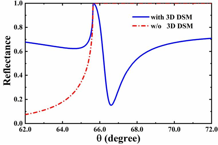
Fig. 2. Comparison plot of reflectance with incident angle with (blue line) and without 3D DSM (red line).
