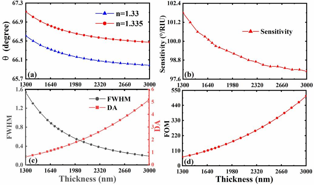
Fig. 4. The incident angle corresponding to the reflected peak (a), sensor sensitivity (b), FWHM and DA (c), FOM (d) with different thickness of 3D DSM.
