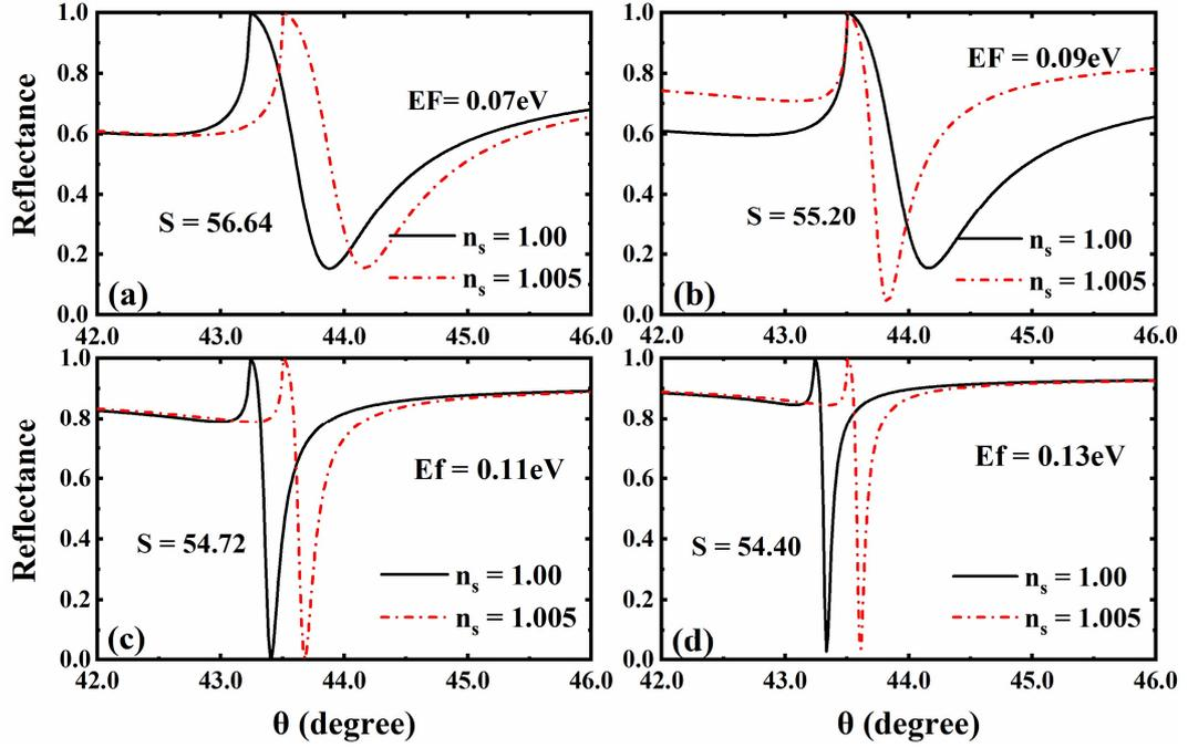
Fig.6. Curve of the reflectance with the angle of incidence at the Fermi energy of the 3D DSM  $E_F = 0.07$  eV (a),  $E_F = 0.09$  eV (b),  $E_F = 0.11$  eV (c),  $E_F = 0.13$  eV (d), respectively.
