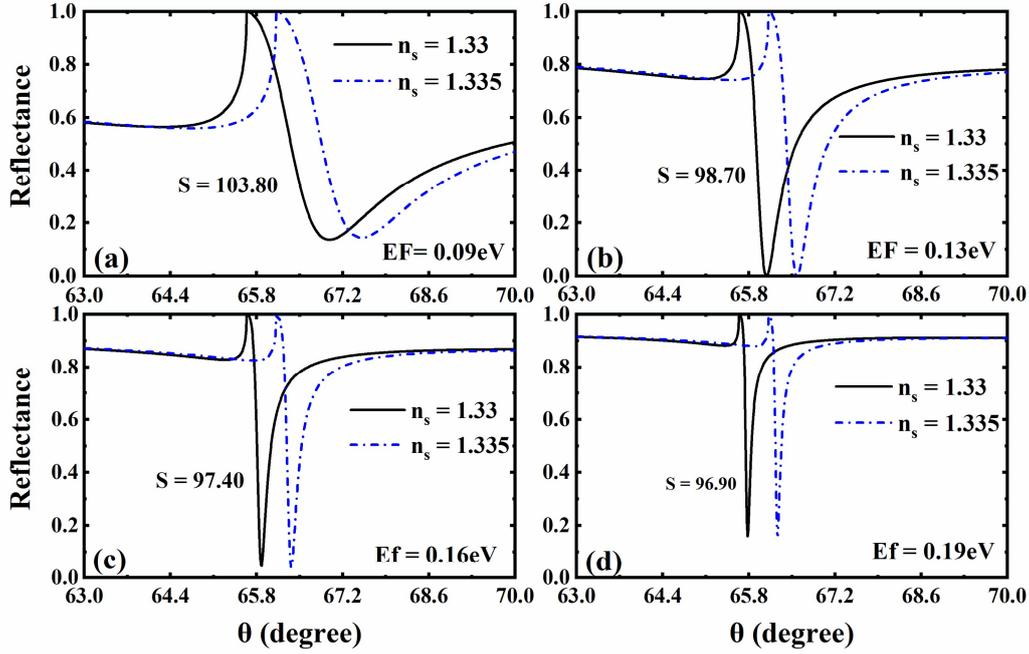
Fig.5. Curve of reflectance as a function of incident angle when the Fermi energy of 3D DSM is taken as  $E_F = 0.09$  eV (a),  $E_F = 0.13$  eV (b),  $E_F = 0.16$  eV (c), and  $E_F = 0.19$  eV (d), respectively.
