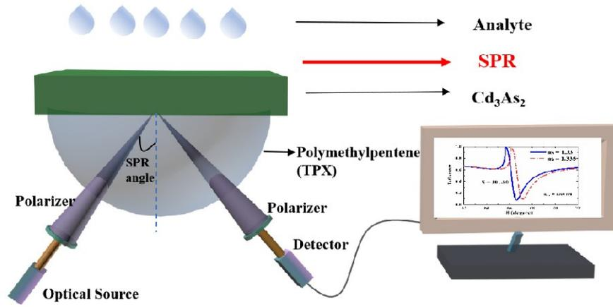
Fig. 1. Schematic representation of SPR sensor based on coupling prism and 3D DSM.
