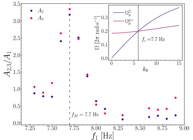
FIG. 10. Normalized amplitudes of the two daughter waves for different frequencies of the mother wave  $f_1$ . We clearly observe a peak at around  $f_M \approx 7.7$  Hz, where the daughter waves are three times larger than the mother wave in amplitude. Inset: Predicted group velocity of the sloshing mode (blue) and phase velocity of gravity-capillary mode (red), intersecting at  $k_c = 6$  corresponding to the peak frequency  $f_M = 7.7$  Hz.
