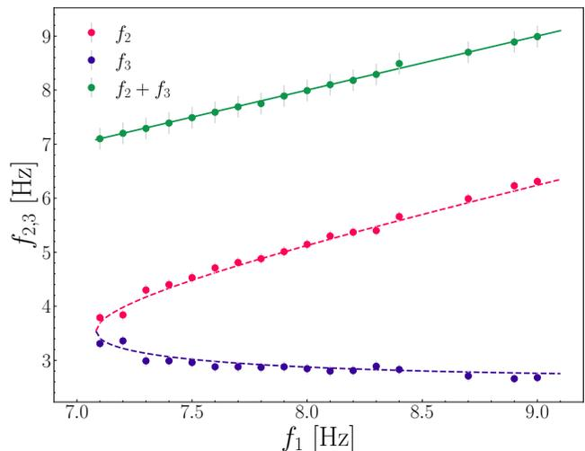
FIG. 7. Measured values (dots) of the daughter frequencies  $f_2$  (red) and  $f_3$  (blue) for different mother frequencies  $f_1$ . The dashed lines are theoretical values obtained numerically through the resonance conditions of Eq. (4). Solid line of slope 1 corresponds to  $f_1$  and green dots indicate the sum  $f_2 + f_3$ .
