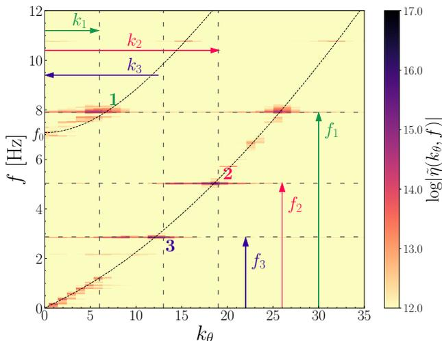
FIG. 5. Fourier spectrum  $\tilde{\eta}(k_\theta, f)$  of the torus outer border displacement  $\eta(\theta, t)$ . Monochromatic forcing at  $f_1 = 7.9$  Hz. Points  $(k_2, f_2)$  and  $(k_3, f_3)$  lie on the gravity-capillary branch whereas, point  $(k_1, f_1)$  lies on the sloshing branch where it is forced. All three points verify the resonance conditions in both frequency and wavenumber (see arrows).  $f_0$  is the cutoff frequency of the sloshing branch.
