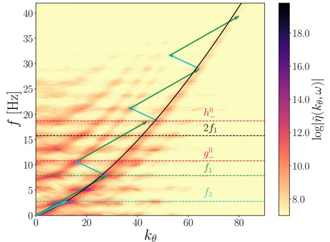
FIG. 12. Fourier spectrum  $\tilde{\eta}(k_\theta, f)$  of the torus outer border displacement  $\eta(\theta, t)$ . Most of the energy is concentrated along the gravity-capillary branch. Quasiresonant interaction is observed following Eq. (17) and Eq. (18) with  $\delta k_\theta = 1.6$ . Monochromatic forcing at  $f_1 = 7.9$  Hz.
