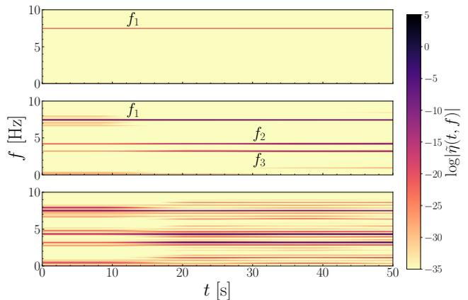
FIG. 4. Time-frequency spectrum of the wave amplitudes of Fig. 3. For low forcing, a single frequency is present,  $f_1 = 7.4$  Hz (top), but for a high enough forcing, two frequencies appear at  $f_2 = 4.2$  Hz and  $f_3 = 3.2$  Hz (middle). Further increase of the forcing generates an ensemble of different modes (bottom).
