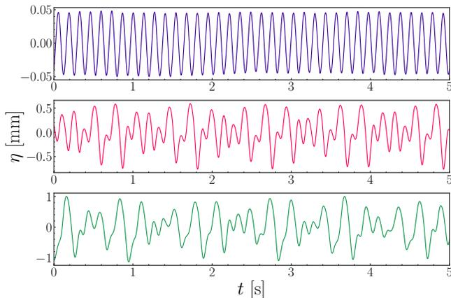
FIG. 3. Displacement  $\eta(t)$  at a fixed point for three different amplitudes of forcing ( $f_1 = 7.4$  Hz) increasing from top to bottom with the corresponding values of wave steepness  $\epsilon = 0.003, 0.02, \text{ and } 0.03$ . The signal goes from a sine wave into a superposition of various subharmonics.
