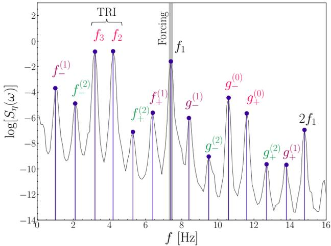
FIG. 11. Power spectrum of a signal forced at  $f_1 = 7.4$  Hz. The forcing is strong enough to excite additional couples besides the primary three-wave pairs,  $f_1^{(1)}$  and  $f_2^{(1)}$ . The first two daughters, continue to generate firstly the subharmonic secondary waves of Eq. (15), which then go on to create tertiary waves through interactions with the mother wave at  $f_1$ .
