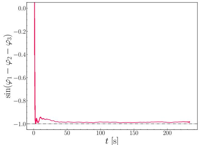
FIG. 9. Temporal evolution of the sine of the total phase  $\varphi = \varphi_1 - \varphi_2 - \varphi_3$  of the three waves obtained using the argument of the Hilbert transform. The total phase  $\varphi$  is found to be locked to a value close to  $-\pi/2$ . Same forcing as in Fig. 8.
