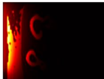
(a) The simulation result of light absorption, which is used as initial pressure distribution.
