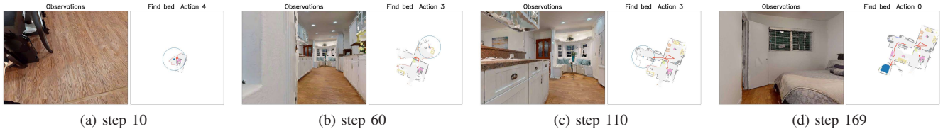
Fig. 5: The visual target navigation experiment process in the Habitat platform for finding a bed. The gray channel represents the barrier, the blue spot and the circle denote the long-term goal selected by our policy, the red thick line represents the trajectory of the robot, the red thin line denotes the frontiers, and other colors represent the semantic objects.
