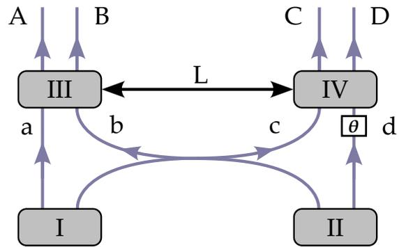
FIG. 4. Proposed experimental setup for observing a nonlocal quantum interference phenomenon of the origins of a photon-quadruple. Here, four photons are created either in crystal I&III or II&IV, with a large distance  $L$  between the crystals which could lead to the observation of the nonlocal features of a multipartite quantum system. The experiment has been proposed in [4, 12] and recently demonstrated for small  $L$  in [9, 11].
