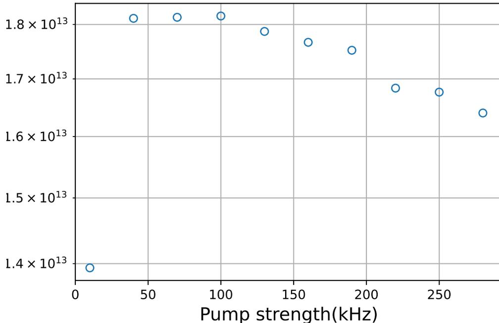
FIG. 5. The steady-state number of photons as a function of the optical pump strength, defined by Eq. (1), at high pump strengths. For the parameters listed in Table I, the number of microwave photons begins to decrease if the pump strength is increased beyond around 100 kHz because the  $\text{NV}^-$  centres begin to accumulate in the  $|7\rangle$  state due to its slow decay rate. This tends to reduce the population inversion and inhibit maser action.
