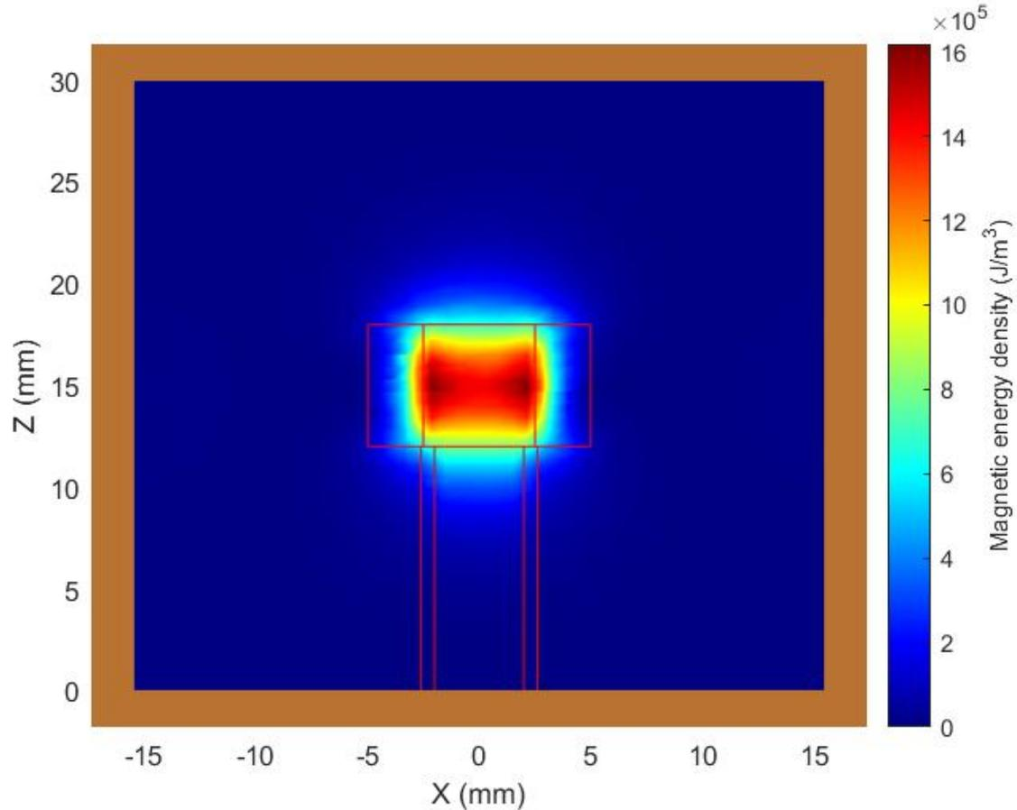
FIG. 2. The energy density of the magnetic field of the  $TE_{01\delta}$  mode of a cylindrical copper cavity simulated using CST Microwave Studio. The red outlines show the boundaries of a sapphire resonator and post. The walls of the copper cavity are shown as the enclosure that bounds the image.
