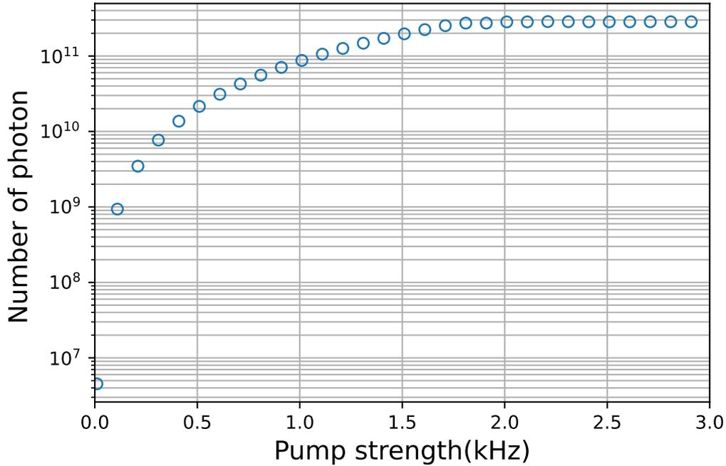
FIG. 4. The steady-state number of photons as a function of the optical pump strength, defined by Eq (1), at low pump strengths. For the parameters listed in Table I, the photon number saturates at a pump strength of around 1.5 kHz.
