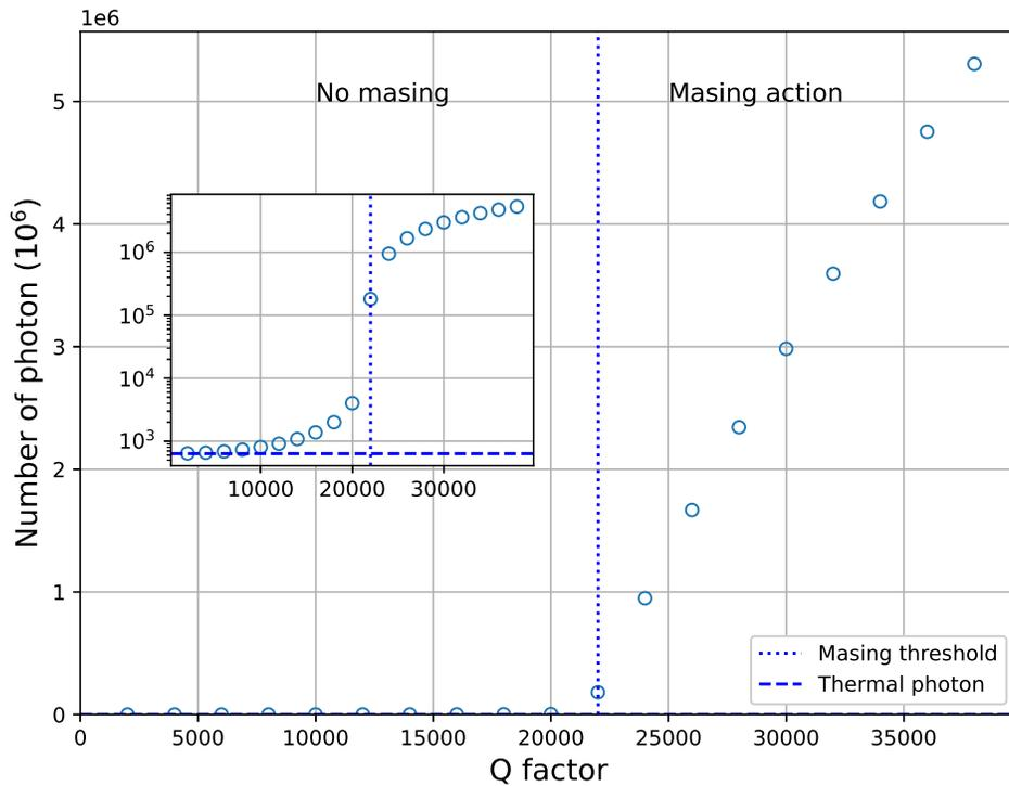
FIG. 3. The steady-state number of photons as a function of the loaded cavity  $Q$  factor. The photon number shows threshold behaviour with respect to the  $Q$  factor, with the onset of masing at around  $Q = 22000$  for the parameters listed in Table I. The inset shows the onset on a logarithmic scale.
