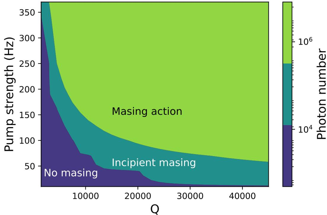
FIG. 7. The steady-state microwave photon number as a function of the optical pump strength and the loaded cavity Q-factor. We identify a masing regime, a non-masing regime and an intermediate “incipient masing” regime in which stimulated emission dominates spontaneous emission, but the maser cannot achieve self-sustaining oscillations. At all pump strengths, the photon number increases monotonically with the Q-factor as expected.
