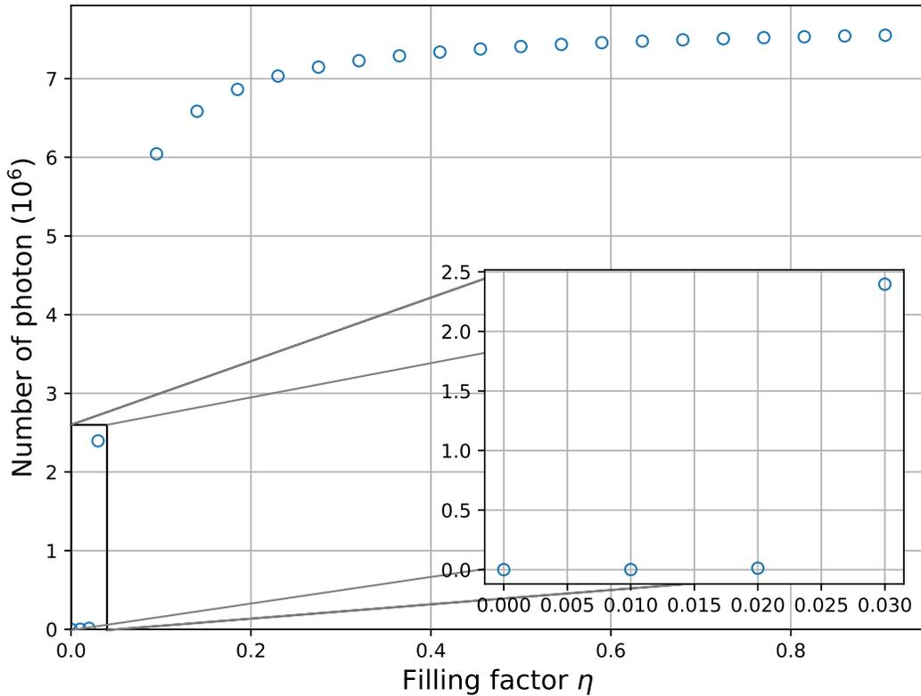
FIG. 8. The number of microwave photons in the cavity as a function of the filling factor, defined by Eq. 4. The number of photons becomes saturated above  $\eta = 0.3$ . The inset shows the onset of masing at a filling factor of 0.03.
