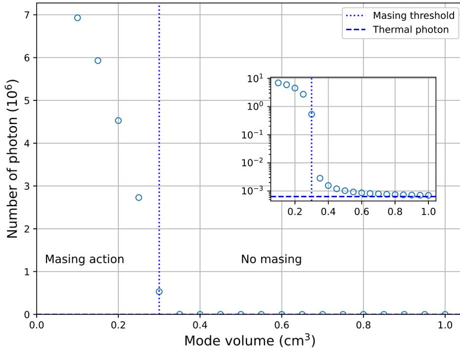
FIG. 6. The steady-state number of microwave photons as a function of the cavity mode volume for the parameters listed in Table I. The masing threshold occurs at a mode volume of about  $0.3 \text{ cm}^3$ . The inset shows the onset on a logarithmic scale.
