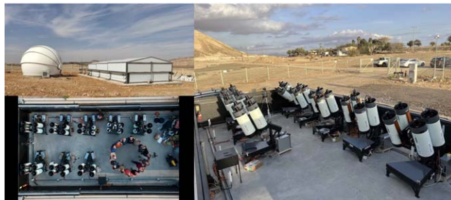
Figure 2. From left and clockwise: The LAST rolling roof enclosure; Panoramic view of the LAST 32 telescopes currently installed. The remaining 16 telescopes will be installed in summer 2023; Top view of the LAST enclosure.
