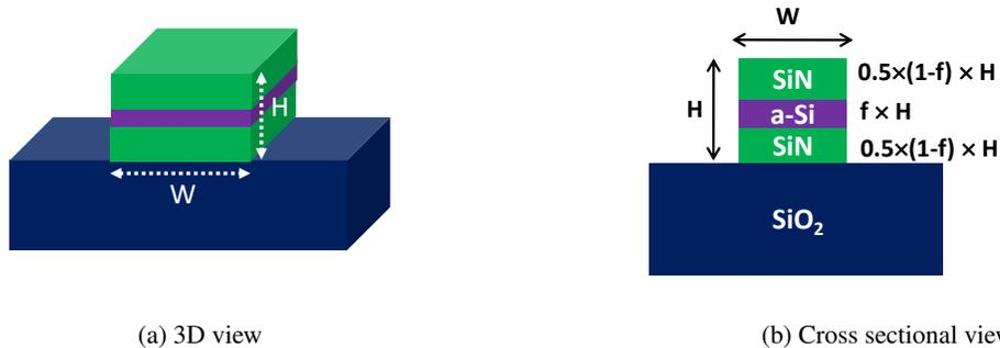
Figure 1: Schematic of the hybrid sandwich waveguide (a) 3D view and (b) Cross-sectional view showing various design parameters of waveguide.
