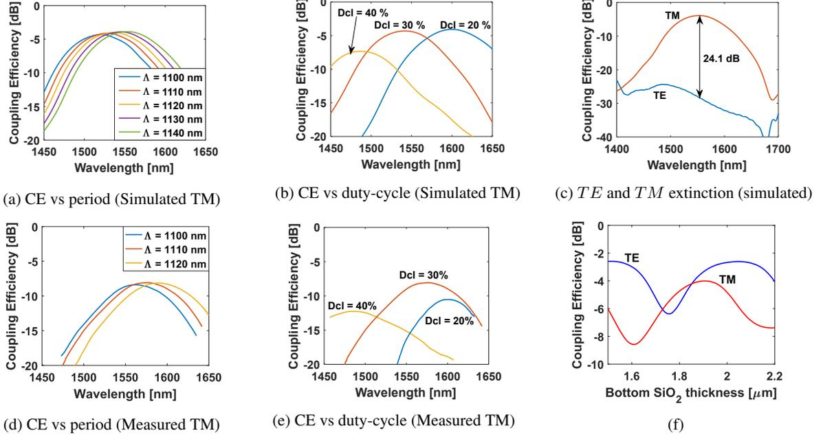
Figure 9: Summary of simulation and measurement of *TM* grating couplers. Simulated coupling efficiency (CE) of a *TM* gratings to (a) grating period and (b) duty-cycle. (c) Extinction of *TM* and *TE* of a *TM* gratings. Measured Coupling efficiency of *TM* gratings as a function of (d) etch depth and (e) duty-cycle. (f) Effect of bottom oxide thickness on the CE of *TE* and *TM* gratings.
