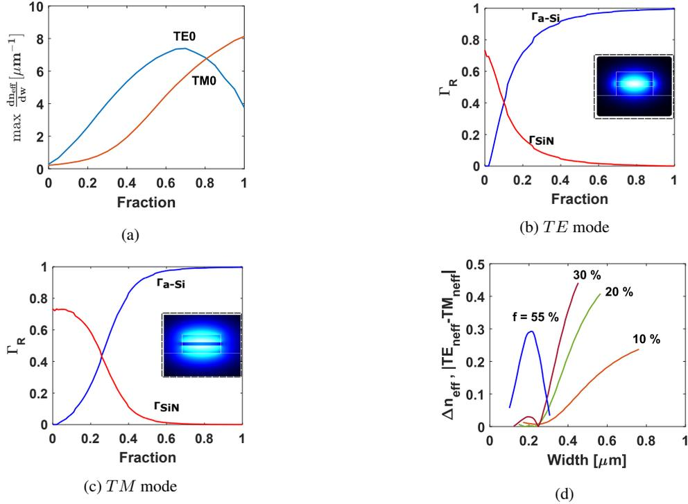
Figure 5: Analysis of oxide clad waveguide. (a) Maximum slope of effective index vs width as a function of fraction. Confinement of (b)  $TE$  mode and (c)  $TM$  mode in  $a-Si$  and  $SiN$  layers as a function of fraction. Inset shows the field for  $TE$  mode for  $f = 20\%$ . (d) Polarization birefringence vs width as a function of fraction.
