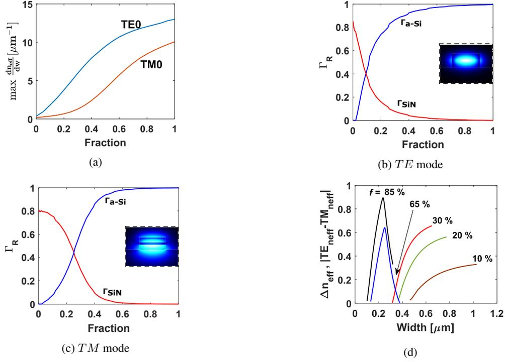
Figure 3: Analysis of air clad waveguide (a) Maximum slope of effective index vs width as a function of fraction. Confinement of (b)  $TE$  mode and (c)  $TM$  mode in  $a-Si$  and  $SiN$  layers as a function of fraction. Inset shows the field distribution for  $f = 20\%$ . (d) Polarization birefringence vs width as a function of fraction.
