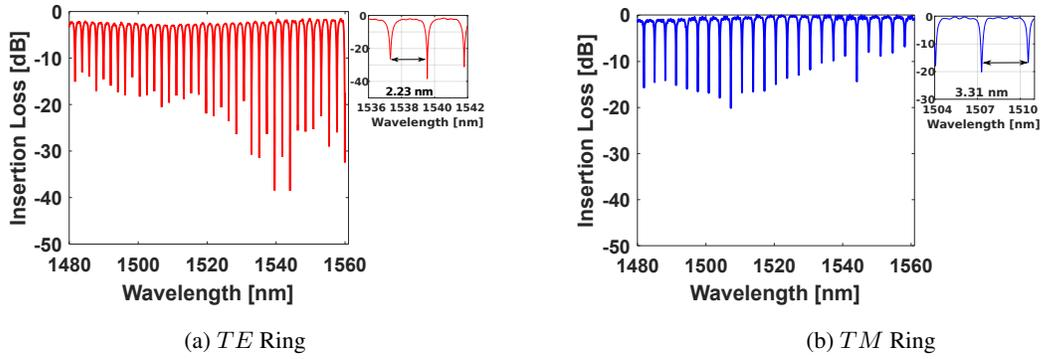
Figure 12: Normalized Spectral response of (a)  $TE$  and (b)  $TM$  ring resonators.
