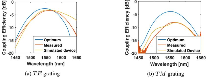
Figure 10: Optimal design and measured coupling efficiency of (a)  $TE$  and (b)  $TM$  grating couplers.
