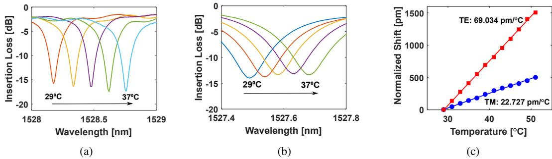
Figure 13: Thermo-optic response of the hybrid waveguide. Spectral shift with temperature for (a)  $TE$  polarization and (b)  $TM$  polarization. (c) Linear thermo-optic response shift for  $TE$  and  $TM$ .
