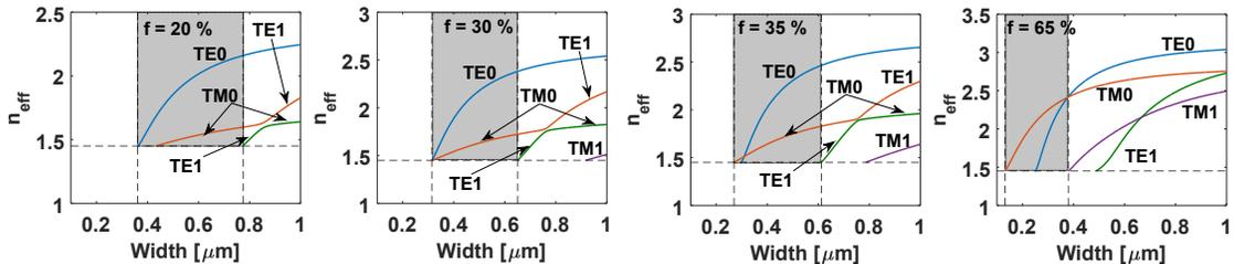
Figure 2: Effective index for various fraction 'f' showing fundamental and higher order modes for air clad. The shaded region shows the single-mode regime.
