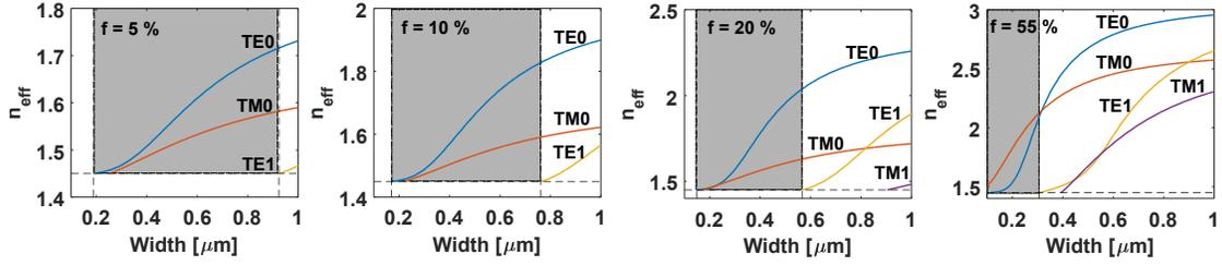
Figure 4: Effective index for various fraction  $f$  showing fundamental and higher order modes for oxide clad. The shaded region shows the single-mode regime.
