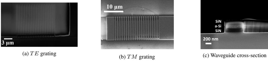
Figure 7: SEM image of a fabricated (a) TE grating in  $a-Si$  layer, (b) top view of full stack etched TM grating, and (c) cross-section of 700 nm wide and 20% fraction fabricated waveguide showing the three layers.
