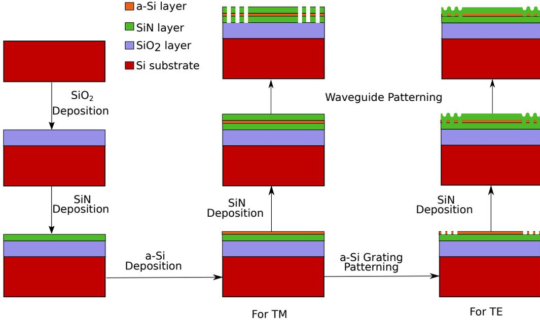
Figure 6: Overview of  $TE$  and  $TM$  grating and waveguide fabrication process flow.
