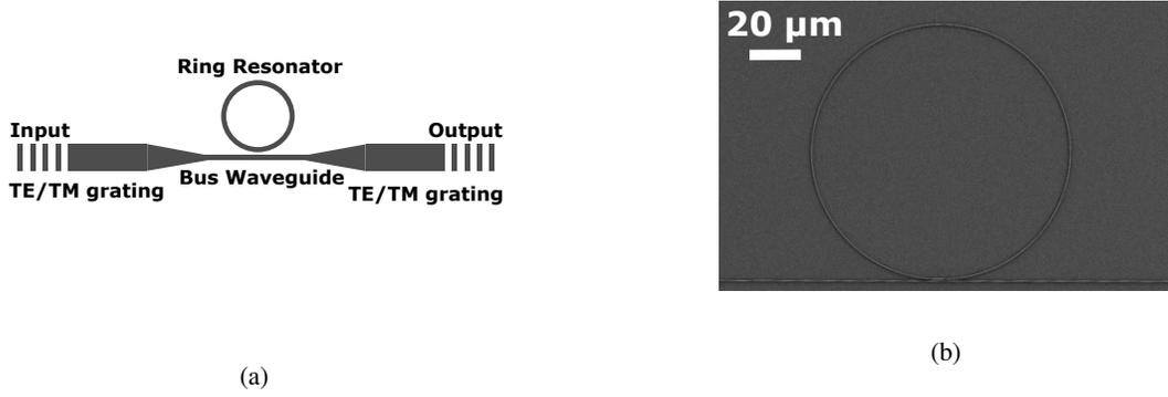
Figure 11: (a) Schematic of the test structure and (b) SEM of the fabricated ring resonator
