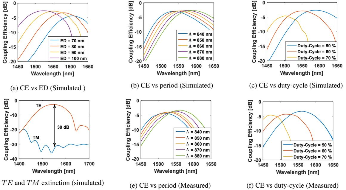
Figure 8: Summary of simulation and measurement of TE grating couplers. Simulated coupling efficiency (CE) of a TE gratings to (a) etch depth of in 100 nm  $a-Si$ , (b) grating period, and (c) grating duty-cycle. (d) Extinction of TM and TE of a TE gratings. (e) Measured spectral response of TE gratings as a function of etch depth. (f) Measured spectral response of TE gratings as a function of duty-cycle.
