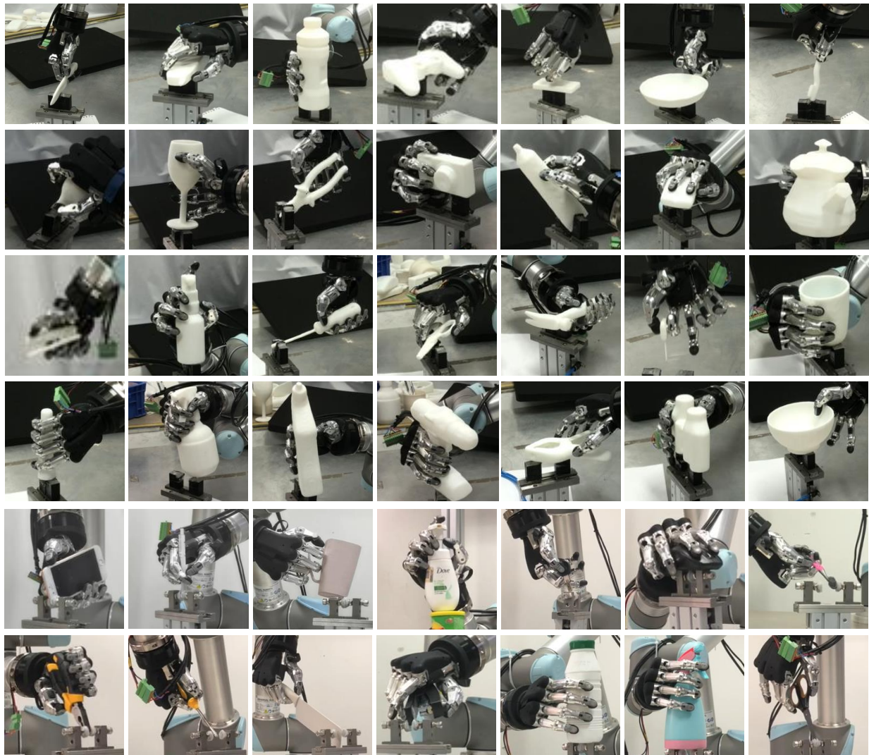
Fig. 21. Functional grasps with 5-Finger Schunk Hand on real robot platform. The first four columns show grasps on 28 3-D printed objects, and the last two columns show grasps on 14 real objects collected from our lab. Best view in color and zoom in.
