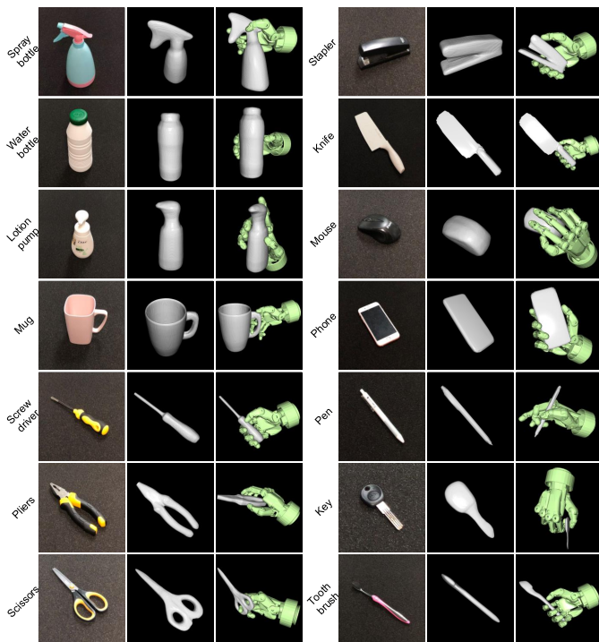
Fig. 16. Qualitative results for shape completion and grasp generation for 14 test objects used in real robot experiments. Best view in color and zoom in.
