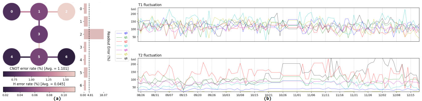
FIG. 2. (a) Error map of ibm_nairobi on Dec. 9, 2022, generated by the IBM Q platform [17]. (b) T_1/T_2 fluctuation of the 7 physical qubits inside ibm_nairobi . 100 data points were collected from Aug. 25 to Dec. 18, 2022. Note that data is not continuous due to scheduled/unscheduled system maintenance, for example around Nov. 1.
