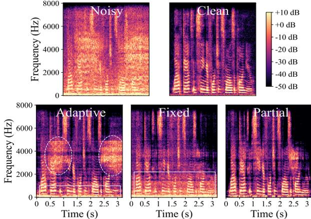
**Fig. 2.** Spectrograms of an audio example. Clean speech is distorted by both ego-noise and environmental noise. The three plots in the second row represent the reconstructed speech spectrograms obtained by three compared methods.
