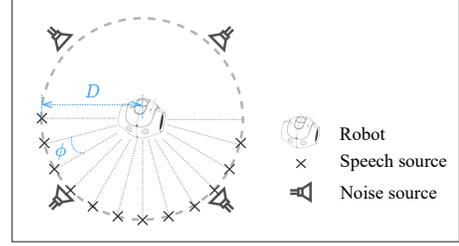
**Fig. 1.** Illustration of the recording setup with the NAO robot [21]. Room dimensions (length  $\times$  width  $\times$  height):  $504 \times 930 \times 284$  cm;  $T_{60} \approx 200$  ms; speaker-robot distance  $D \approx 1$  m;  $\phi \approx 15^\circ$ .
