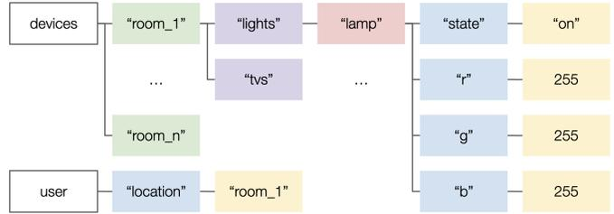
Fig. 1: Data structures for expressing smart home device and user context in prompts to an LLM.
