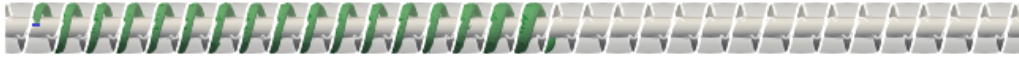
Figure 8. Screw conveyor test case: Illustration of the domain. The fluid is marked in green, and the fluid inlet is marked in blue on the left of the domain. The screw rotates clockwise around its axis, while the casing is fixed. As the screw rotates, the fluid is transported from the left to the right side in the figure.
