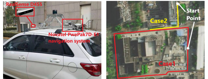
Fig. 7: The vehicle and sensor layout. Fig. 8: The test environment.
