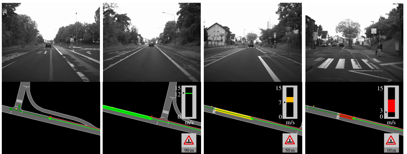
Fig. 10: Regulatory risk example. In the situation, the driver does not let a prioritized pedestrian pass first on the crosswalk. RNS warns of the upcoming traffic object and displays the distance and colors the ego lane according to the risk.
