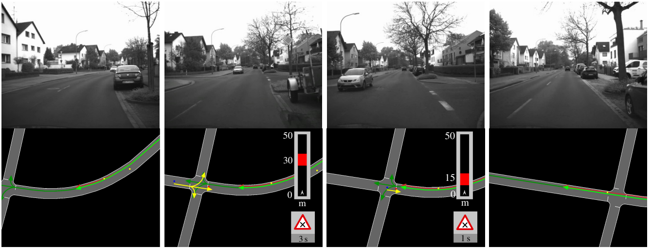
Fig. 8: Collision risk example. At intersections, RNS calculates TTCE for combinations of ego plus other vehicle's path and informs about the critical encounter point (red line: recorded trace from ego car, green line: trace projected on navigation path). Top: Stream of front camera images. Bottom: Screen layout of system.
