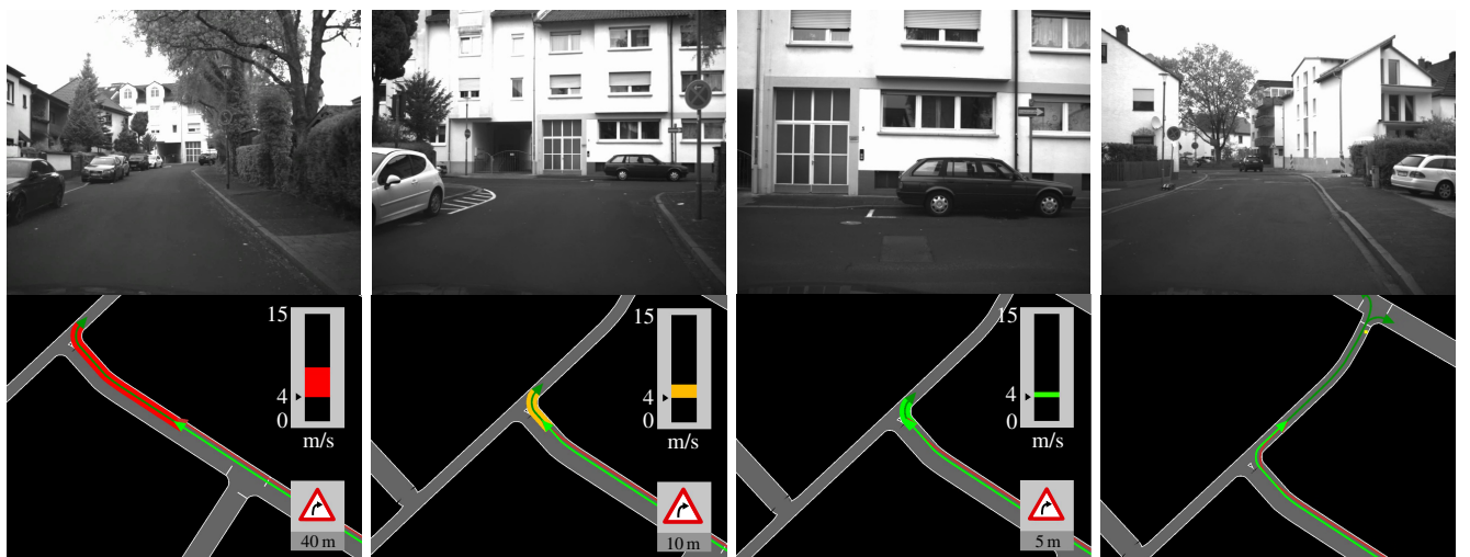
Fig. 9: Curve risk example. RNS detects a sharp turn and recommends to decrease the velocity, which the driver is shortly after abiding to. The velocity scale goes from red (difference of actual to desired velocity) to green (small difference).
