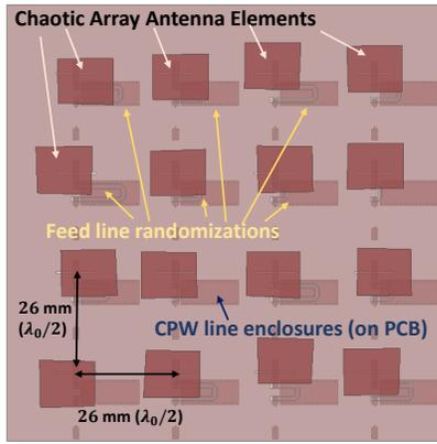
Fig. 1. Ansys model of a 4×4 5.8 GHz ISM band CAA with randomized antenna positions, shapes, and feed line lengths.
