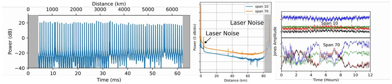
Figure 2: (a) Measured trace from the submarine cable. (b) Zoom-in for intensity measurements from span 10 and span 70. The average time is 60 seconds. (c) All Jones components from the same spans.
