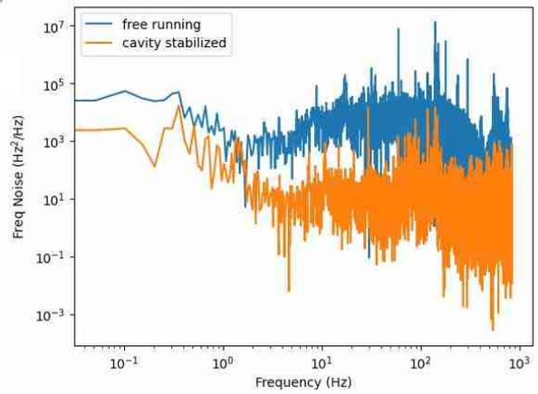
Figure 6: Comparison of frequency noise between a free-running NKT fiber laser and the cavity-stabilized laser system. The distance is about 400km. For frequencies below 1Hz, an improvement of around 10dB is observed, which increases to about 20dB for frequencies between 10Hz to 1kHz.
