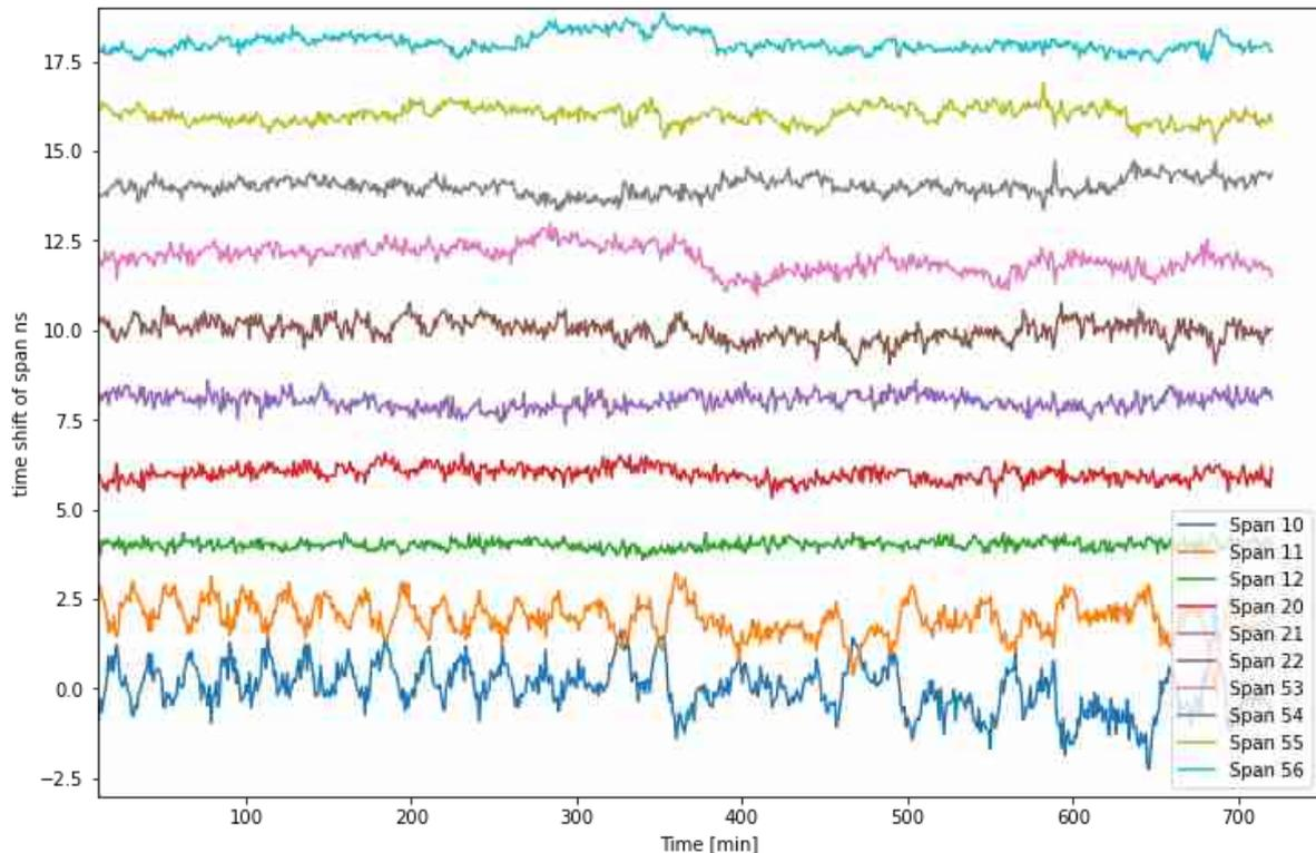
Figure 7: Relative movement of different spans in ns extracted by monitoring the position of each grating. This monitor technique enables identification of cable movement. Looking at span 10-11, we observe highly correlated but opposite direction movement of the two repeaters.
