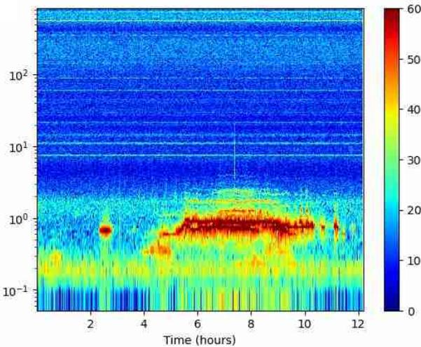
Figure 5: Spectrogram of the phase from span 6. Oscillations observed from 0.1Hz up to a few Hz observed around hour 5-10 are in line with previous observations using polarization measurements from coherent transceivers.
