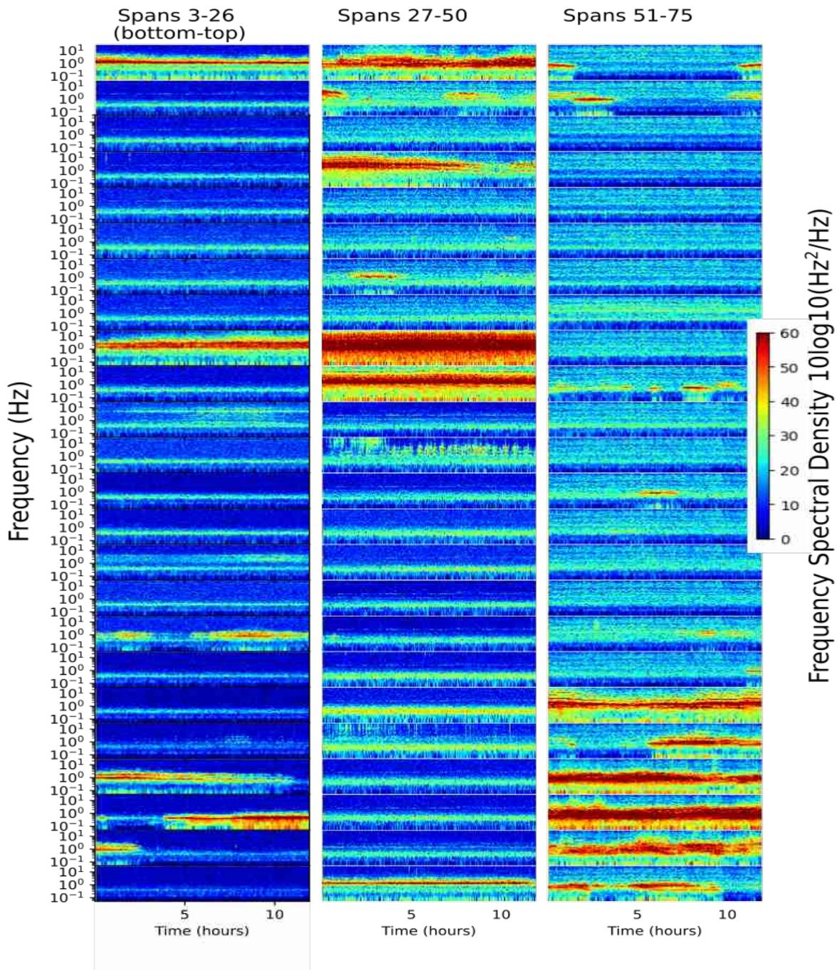
Figure 4: Spectrograms showing the different spans over a 12h measurement time period covering 0.1 to 10Hz.
