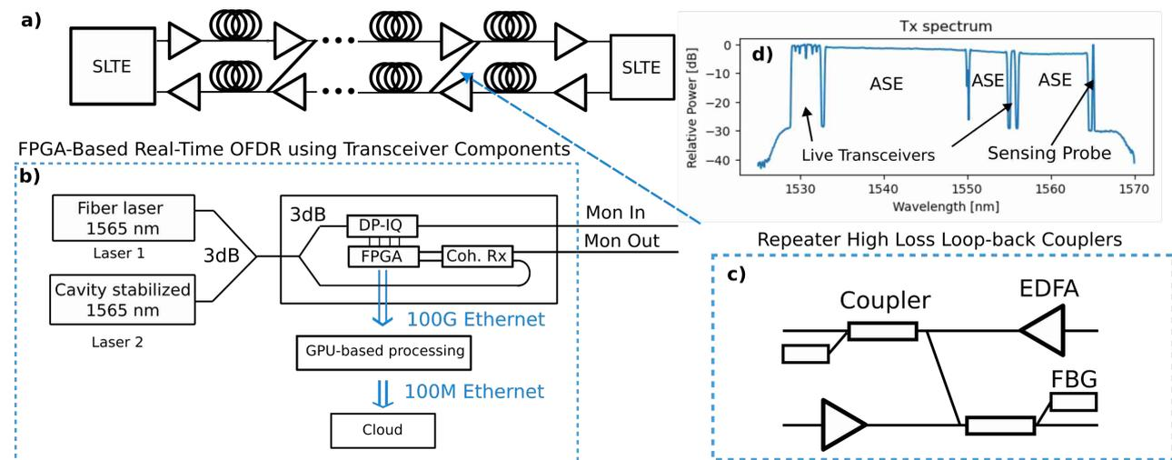
Figure 1: (a) Schematic of a submarine transmission cable system using loop-back connections for monitoring. (b) Block diagram of the coherent continuous power dual-polarization sensing system. (c) Schematic of the high loss loop-back couplers present in each repeater. (d) Transmitted spectrum showing the probe signal out of band.
