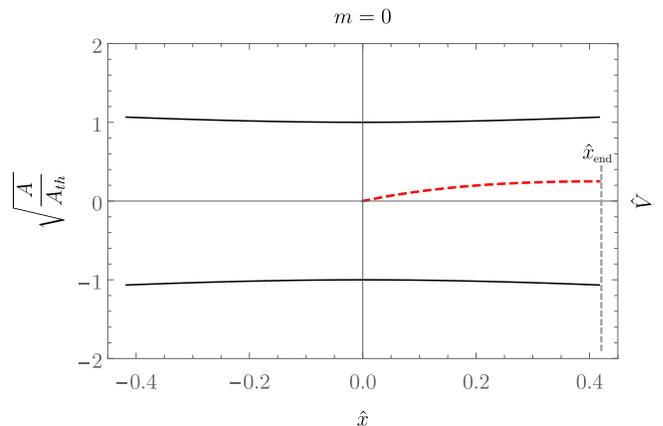
FIG. 1. (Black curve) Lateral section of the Laval nozzle corresponding to the conformally coupled scalar field. The region  $\hat{x} > 0$  ( $\hat{x} < 0$ ) corresponds to subsonic (supersonic) flow. The sonic point (where the fluid velocity equals the sound velocity) is located at the throat  $\hat{x} = 0$ . (Red dashed line) Nondimensional effective potential for acoustic waves in the subsonic region.
