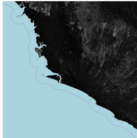
Figure 2: Showing the difference in terrain ruggedness index (TRI) as calculated by the gdaldem tri command between GDAL versions 3.2 and 3.3. The difference would ideally be zero (all black).
