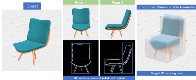
Fig. 3: Each camera individually captures the object (as shown on the left) and computes different regions on the entire geometry. Bounding boxes are fitted to the regions respectively (as shown in the center). Finally, all the bounding boxes are merged from each drone view to form a 3D box (as shown on the right).
