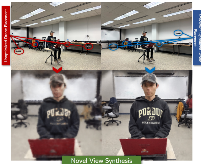
Fig. 1: Comparison of 3D reconstructions with different flight configurations - The left half shows the drones in a conventional circular pattern with no priority to object geometry. The right half shows the optimized position of the drones with a focus on the top half of the person. As a result, the drone facing the person has a higher height compared to the rest of them.
