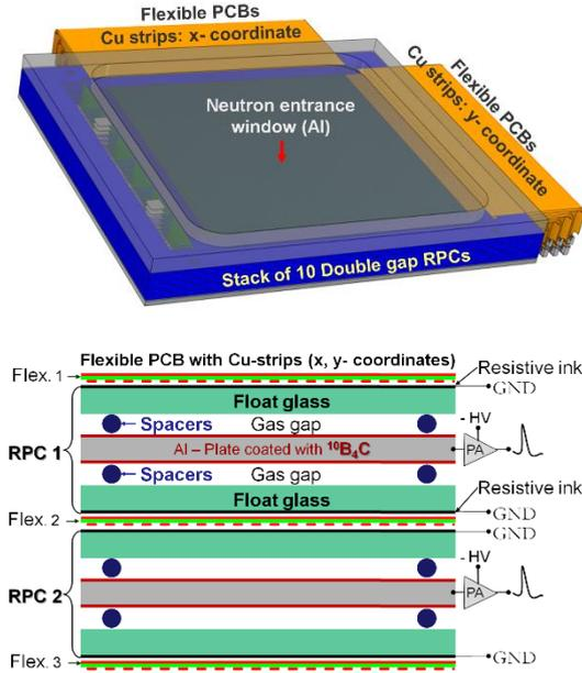
Fig. 1. At the top is a 3D view of the prototype, consisting of a stack of 10 double gap RPCs coated with  $^{10}\text{B}_4\text{C}$ . At the bottom is a schematic drawing (dimensions are not to scale) illustrating the RPCs design, and how the stack is formed (only two RPCs are shown).
