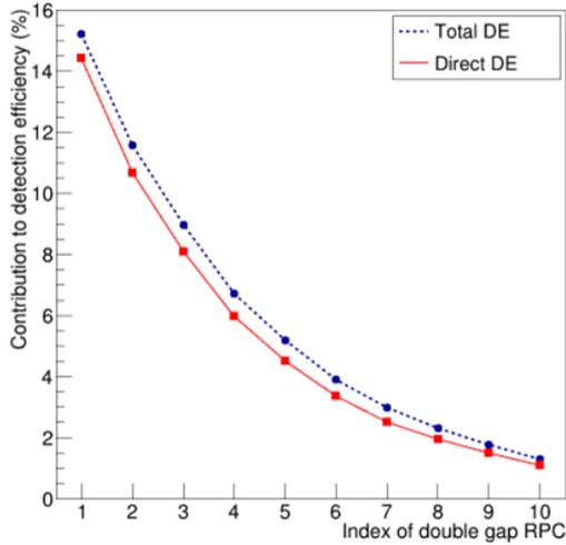
Fig. 2. Contribution to the overall detection efficiency of each double gap RPC in the stack, with  $^{10}\text{B}_4\text{C}$  layers of the same thicknesses ( $1.15\ \mu\text{m}$ ). The sum of all contributions adds up to a detection efficiency of 60.4%. The “direct DE” data show the detection efficiency excluding those neutrons which had prior elastic scattering. The lines are an eye-guide connecting the data points.
