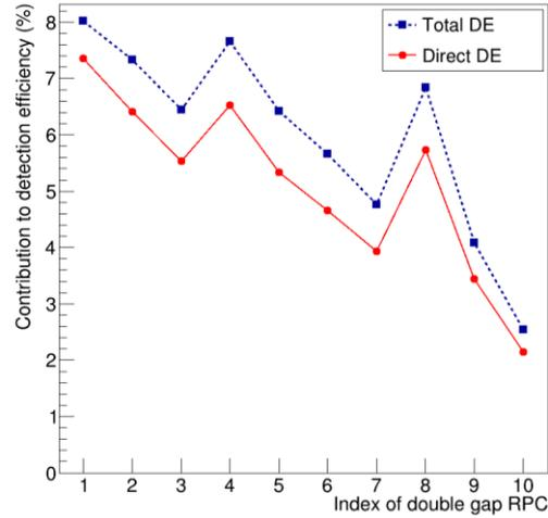
Fig. 3. Contribution to the detection efficiency of each double gap RPC in the stack for the configuration with optimized thicknesses. The sum of all contributions adds up to 59.8% total detection efficiency. The “direct DE” data show the detection efficiency excluding those neutrons which had prior elastic scattering. The lines are an eye-guide connecting the data points.
