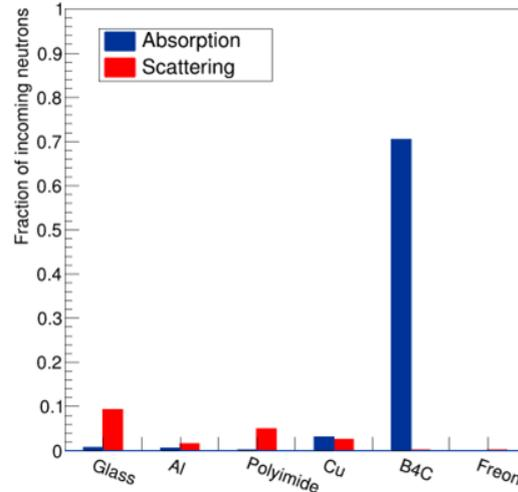
Fig. 5. Fractions of the primary neutrons in the beam lost due to absorption and elastic scattering in all materials of the detector components.
