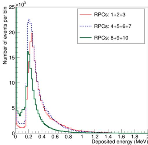
Fig. 4. Distribution of energy deposited in the gas gap, simulated with Geant4 for RPCs with different  $^{10}\text{B}_4\text{C}$  thickness: RPC 1 to 3 of 0.4  $\mu\text{m}$ , RPC 4 to 7 of 0.6  $\mu\text{m}$  and RPC 8 to 10 of 2.2  $\mu\text{m}$ .
