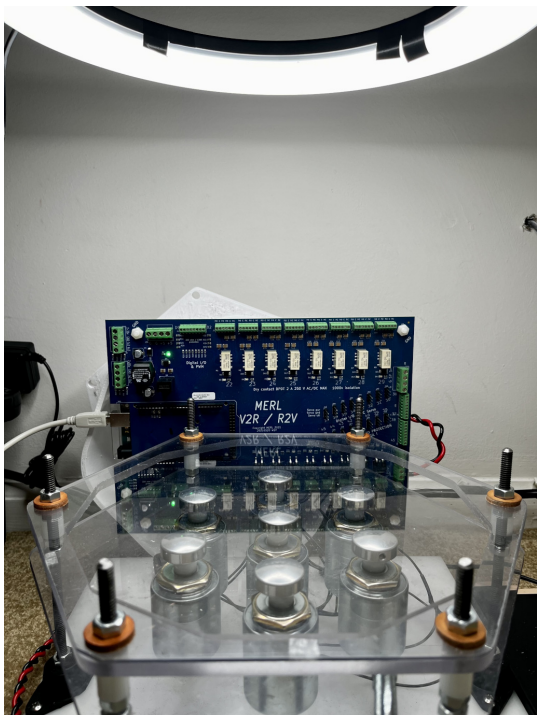
Fig. 1: The 7-solenoid impact manipulation surface "Thumper"; the seven solenoids beneath the transparent support surface are in the foreground, with the controller board in the background
