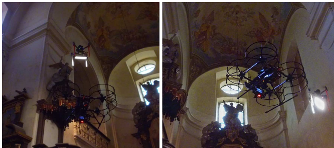
Fig. 2: Deployment of the proposed system for autonomous RTI by a team of UAVs in Church of St. Mary Magdalene in Chlumín. Multimedia material of the experiment is available at http://mrs.felk.cvut.cz/papers/rti2020ral .
