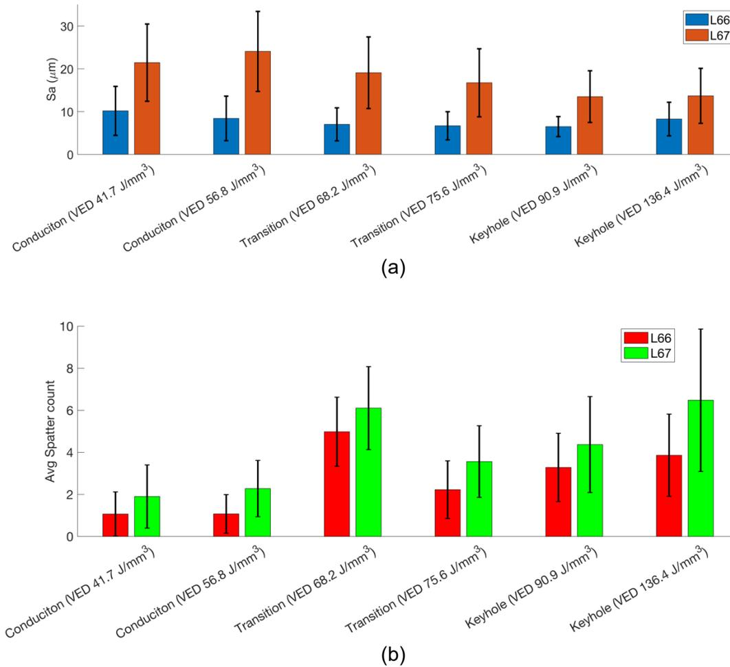
Figure 12. Surface roughness (a) and registered average spatter count per melt pool with one standard deviation (b) for Layer 66 and Layer 67. The error bar in (a) represents one standard deviation of  $Z(x, y)$ , which is the difference between the voxel height at profile coordinates  $x$  and  $y$  and the mean value as shown in Eq. (4).
