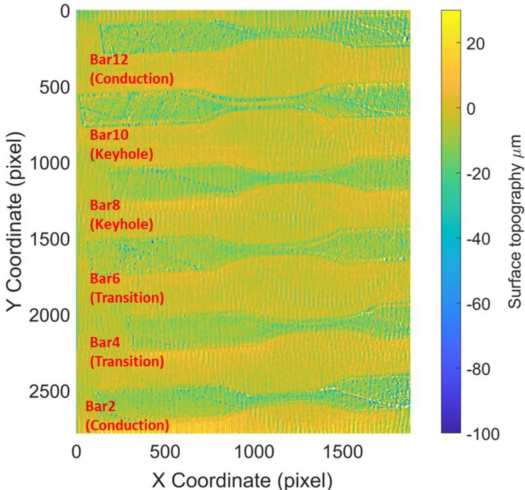
Figure 10. In-situ FPP measured surface topography of in-process Layer 66 of Fatigue Bars 2, 4, 6, 8, 10 and 12 as marked in Figure 1. Note the zero plane is the powder bed surface.
