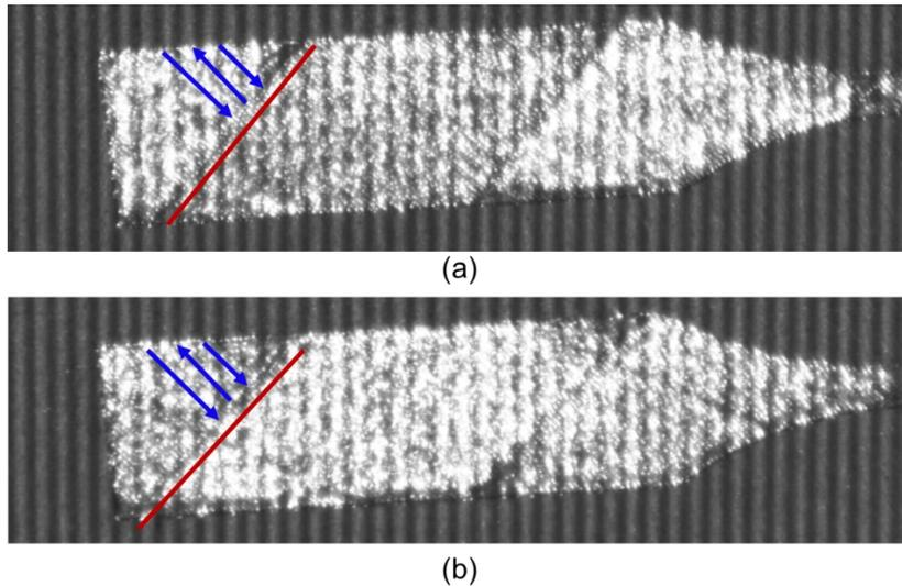
Figure 16. Fringe projection profilometry acquired images for Layer 67 (a) and Layer 75 (b). The hatch strip overlapping is annotated as red line and blue arrow is the laser scan pattern
