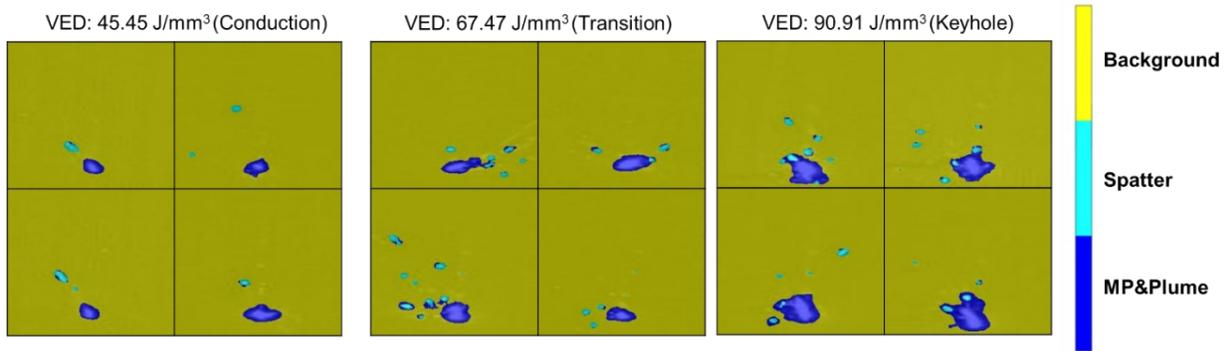
Figure 7. Representative segmentation results of four off-axis camera monitored images are shown for each of the three distinct LPBF process regimes (conduction, transition, keyhole).
