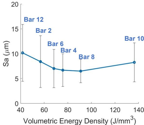
Figure 11. Surface roughness of in-process Layer 66 of the fatigue testing bars measured by the in-situ fringe projection profilometry against the corresponding processing regime’s volumetric energy density. The error bar represents one standard deviation of  $Z(x, y)$ , which is the difference between the voxel height at profile coordinates  $x$  and  $y$  and the mean value as shown in Eq. (4).
