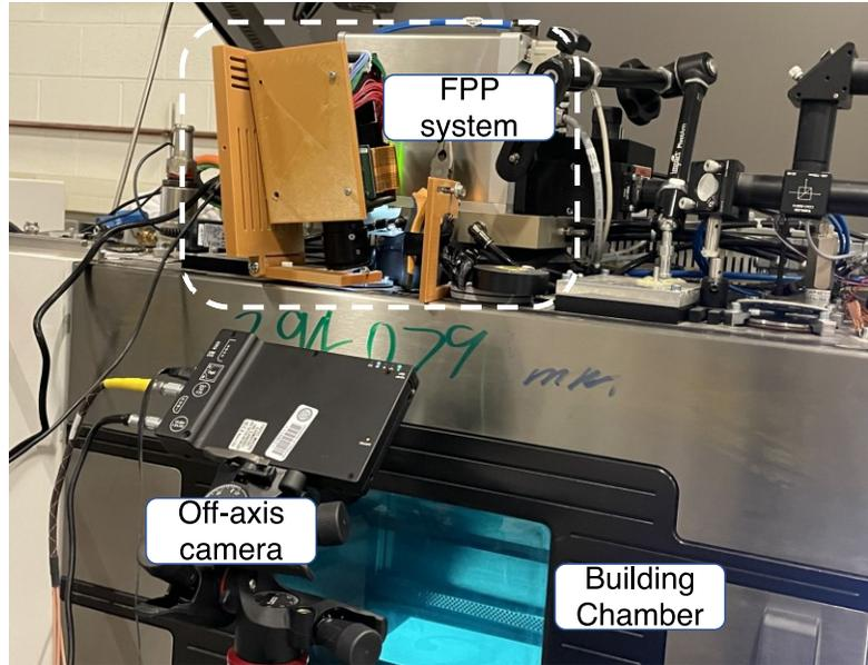
Figure 2. Our in-situ LPBF process monitoring system that integrates an off-axis camera and an in-house fringe projection profilometer for measuring the spatters and layer surface, respectively.
