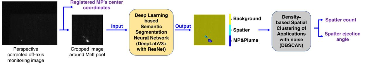
Figure 5. Flowchart of spatter features extraction and registration using off-axis camera-based in-situ monitoring data
