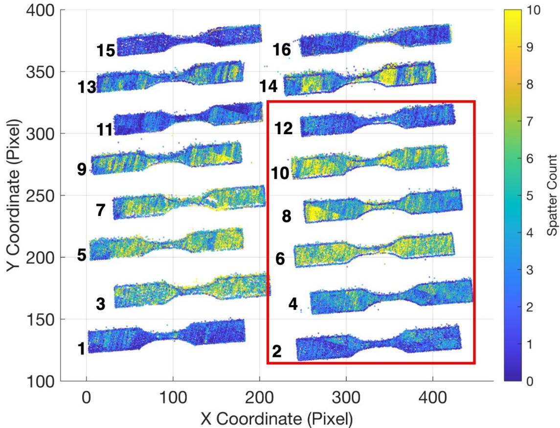
Figure 9. Representative result of spatter signature registration: the registered spatter count at each monitored melt pool in Layer 75 of all the 16 printed fatigue bars. The annotated numbers correspond to the processing parameters in Table 1. All the bars enclosed in the red box are monitored during the printing process by our in-situ Fringe Projection Profilometry and used for surface topography analysis and spatter-roughness correlation in subsequent sections.
