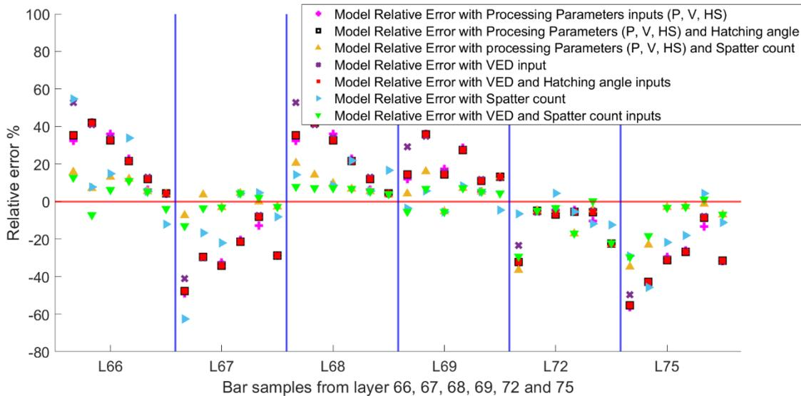
Figure 17. Relative error of the trained models using different combinations of features (process parameters and spatter signature) as predictors to predict the in-process layer surface roughness of six sample layers in six fatigue bars measured by the in-situ FPP. The division of the layers is annotated as the blue vertical line.
