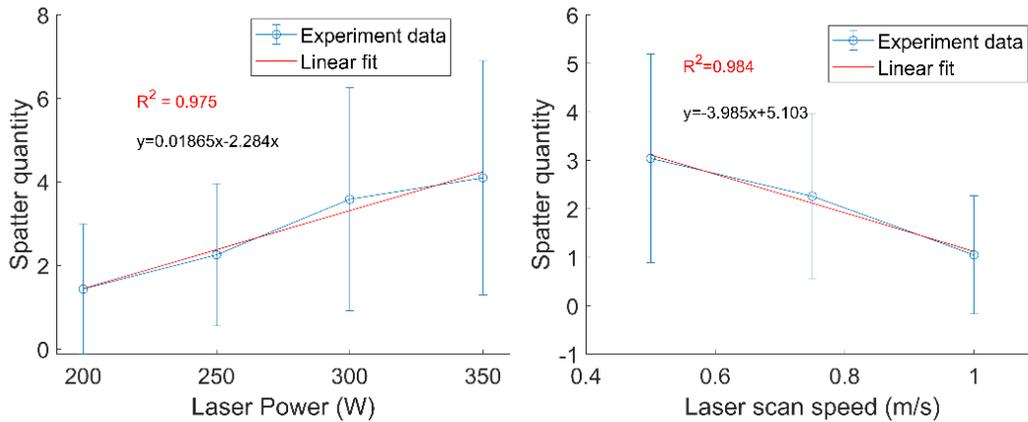
Figure 14. Linear curve fitting of the spatter count (quantity) with the laser power (left) and the laser scan speed (right). The blue circles are the mean values for Layer 66 of the samples printed in the specified parameter and the error bars indicate the standard deviation
