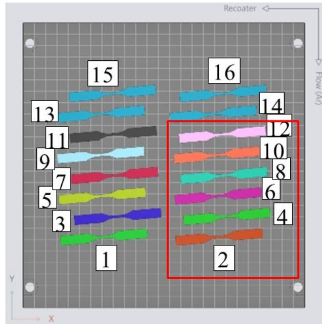
Figure 1. Schematic of our LPBF machine setup for printing 16 fatigue test bars. Bars enclosed in red box are used for surface roughness analysis through Fringe Projection Profilometry
