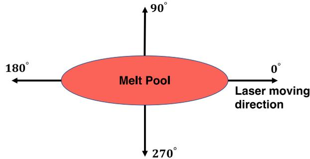
Figure 4. Illustration of the metric of spatter ejection angle
