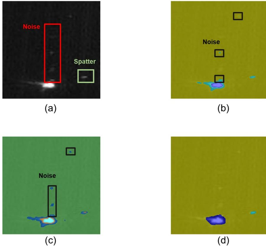
Figure 8. Compare the image segmentation performance of traditional clustering (K-means) and new deep learning-based methods. (a) Raw melt pool image captured by the off-axis camera with actual feature labels. (b) K-means image segmentation (K=3). (c) K-means image segmentation (K=4). Both (b) and (c) falsely classify the noises (e.g., flare artifacts) as spatters. (d) Deep learning (DeepLabV3+ with Resnet) -based Image segmentation used in this work extracts the correct feature of spatter.
