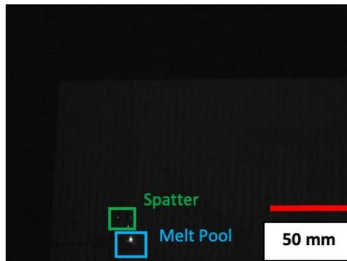
Figure 3. A representative spattering monitoring image captured by our off-axis camera with annotations of melt pool and spatter
