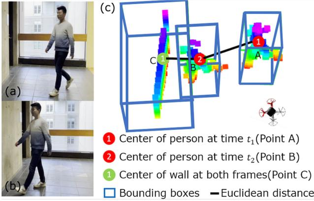
Fig. 6. Illustration of the issue with the center-distance-based data association method. (a) The RGB image at time  $t_1$ . (b) The RGB image at time  $t_2$ . (c) The center-distance-based data association method might fail by incorrectly associating the current detected person with the wall.
