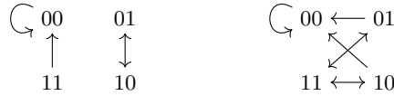
Fig. 2. The synchronous (left) and the asynchronous (right) dynamics of the Boolean network in Example 2.
