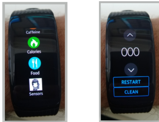
Figure 1: Left: the icon of the sensor application in the Tizen OS menu, right the sensor application with the person-id spinner, restart, and clean button.
