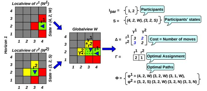
Fig. 4: Cost-optimal goal assignment and optimal paths
