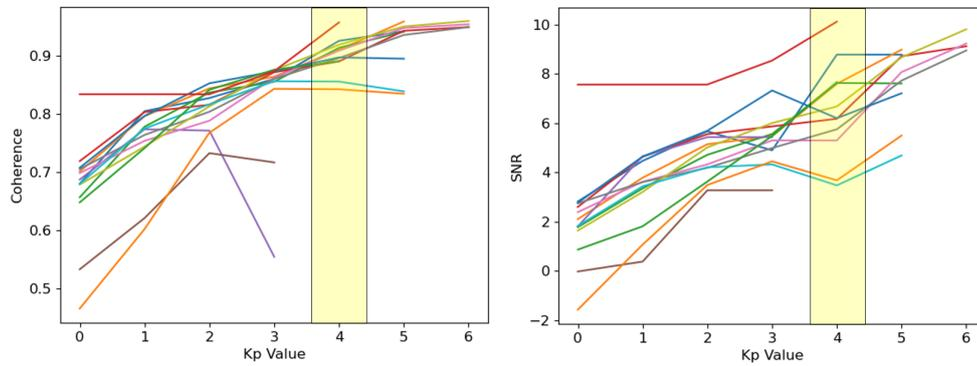
**Fig. 18.** The mean of coherence (left) and SNR (right) comparing measured magnetic field data at newer SWEMDI MT sites with SECS interpolated data (using 3 sites). The SNR and coherence of this comparison is plotted against kp value, highlighting the increase in these metrics with greater magnetic activity. The SNR and coherence of each 3 hour Kp Index bin was recorded, with the mean value plotted.
