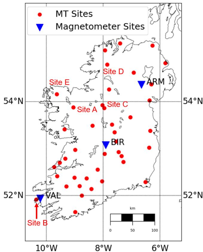
**Fig. 1.** MagIE (ARM, BIR, VAL) magnetometer observatories (blue) and the 43 MT site locations (red) used in this study. Example MT sites (A, B, C, D, E) used subsequently, are marked with red text. Site A was an example site used when optimising a correction for the nowcast geoelectric field. Sites B - E were all used to validate the nowcast model.
