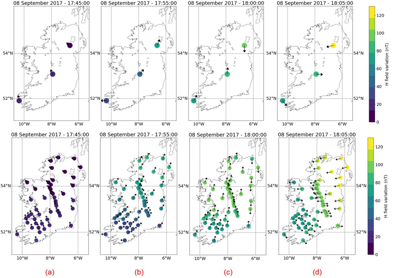
**Fig. 2.** (top) An example of the input magnetic fields at each magnetometer for the 08 September 2017, during an increase in geomagnetic activity. (bottom) The estimated magnetic field at MT sites using a SECS interpolation. At (a) no activity is present. Over time, activity increases from north-east to south-west, with the direction of magnetic fields changing.
