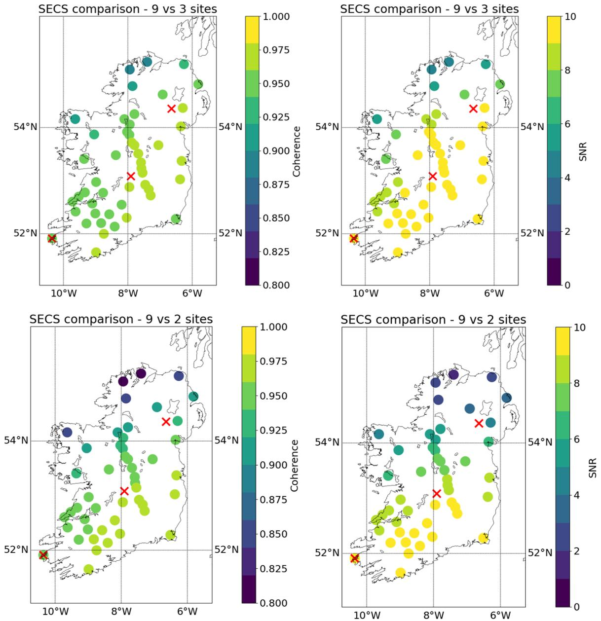
**Fig. 5.** The coherence (left) and SNR (right) between modelled magnetic field using SECS with nine sites is compared to modelled magnetic field using SECS with three magnetometers (top) and two magnetometers (bottom) for the 7-8 September 2017 storm (Kp8). Positions of the MagIE magnetometers are denoted by red crosses.
