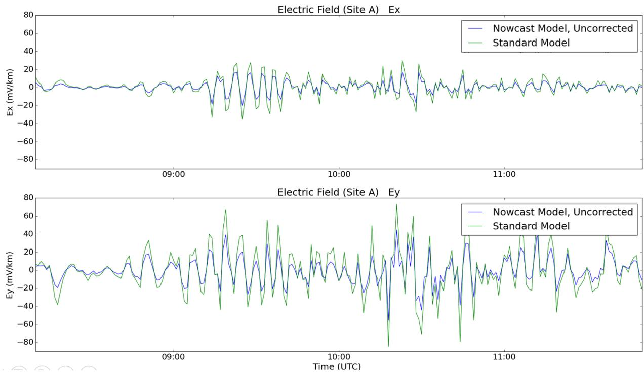
**Fig. 8.** An example of the modelled time series of the electric field at a 1-minute delay (nowcast) plotted against a time series of the standard non real-time model for  $E_x$  (top) and  $E_y$  (bottom) for the 30 October 2003 for Site A (Fig. 1).
