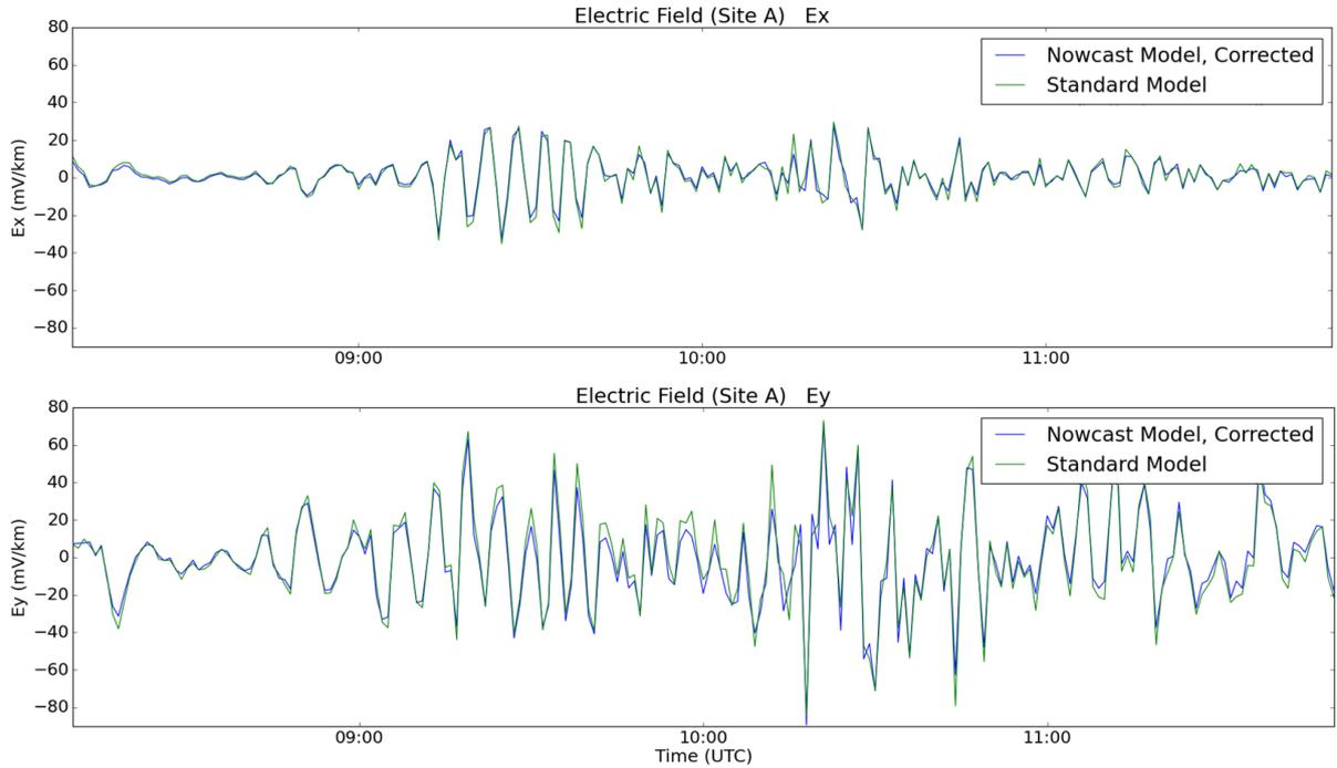
**Fig. 10.** The corrected time series of the electric field at a 1-minute delay (nowcast) against the standard model for  $E_x$  (top) and  $E_y$  (bottom) from Figure 8, with a pre-optimised correction factor of 1.61 (Fig. 9).
