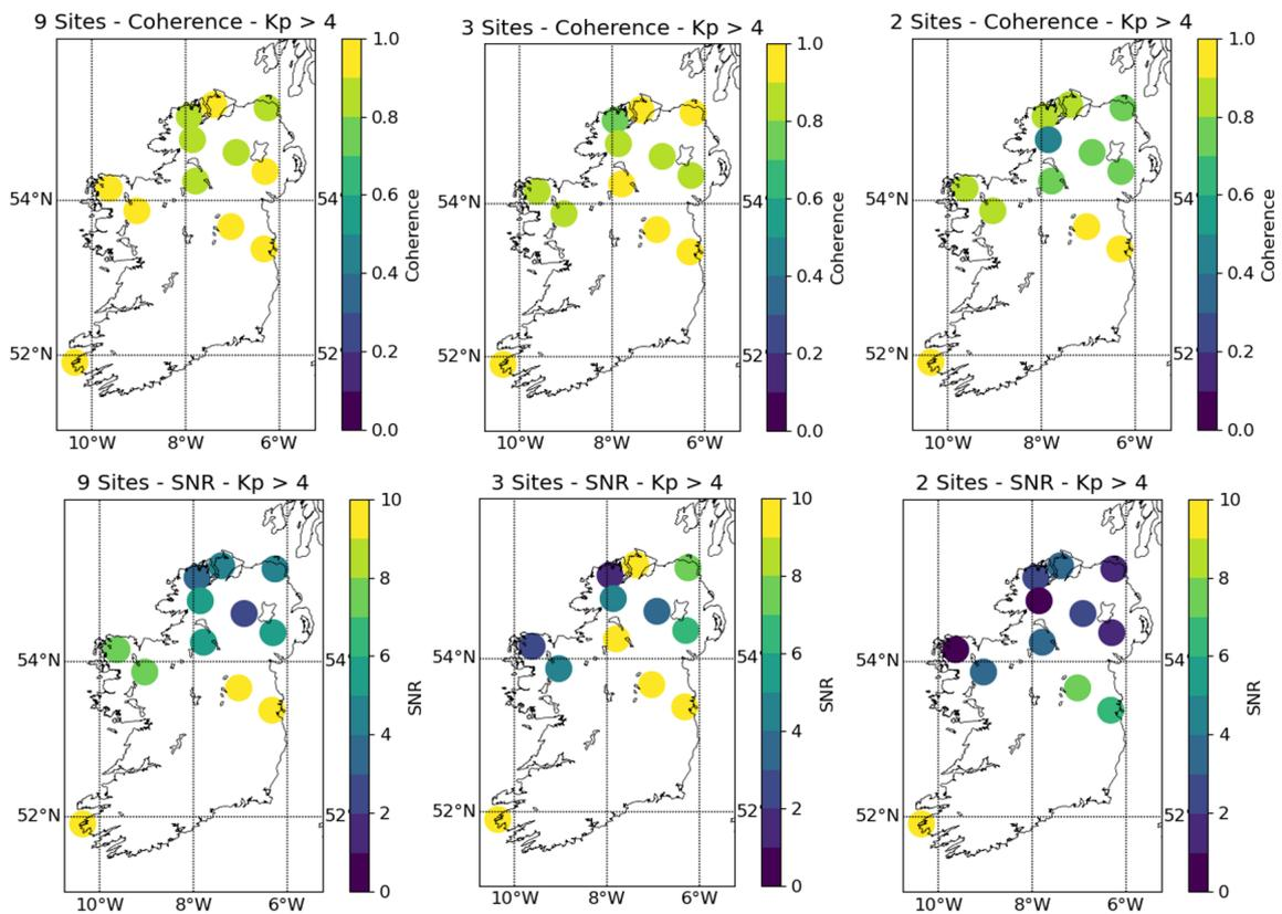
**Fig. 4.** The coherence (top) and SNR (bottom) between the measured magnetic field at MT sites and modelling magnetic fields (SECS interpolation with nine, three and two magnetometer sites) for all MT sites with available data.
