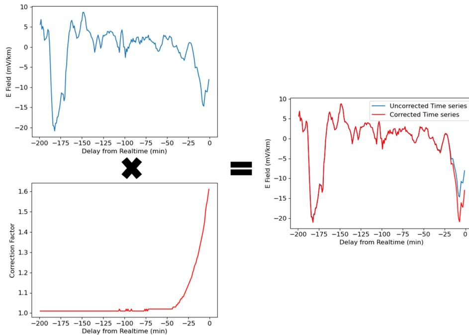
**Fig. 11.** An example of the change in the time series near real time when the electric field time series is multiplied by the correction curve. The uncorrected time series (top left) are multiplied by a correction (bottom left), to give the corrected time series (right).
