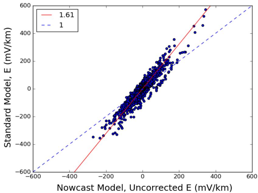
**Fig. 9.** The amplitude of the standard electric field model (both  $E_x$  and  $E_y$ ) are plotted against the corresponding 1-minute delayed from real time (nowcast) electric fields, for all sites in Figure 1 and storms in Table 1. The ideal correction factor (in red) is the best fit slope between the two models and is compared to a slope of unity (in blue).
