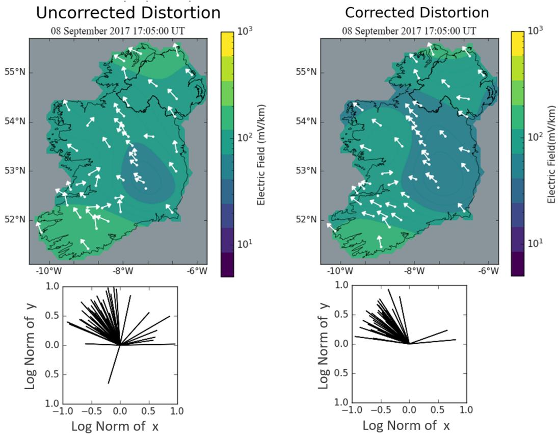
**Fig. 15.** (Top) The model with undistorted electric field (left) is compared to the model with distorted electric field (right). (Bottom) The normalised direction of the vectors above are compared for significantly strong ( $> 5 \text{ mV/km}$ ) electric fields at the same origin.
