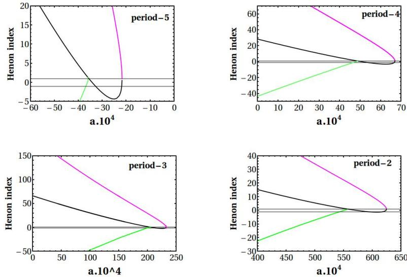
**Figure 11.** The  $HI$  as functions of the parameter  $\alpha$  of the asymmetric orbits of period 5,4,3,2. They all follow the same pattern and they disappear with a tangency at a maximum  $\alpha$  between the stable and a corresponding unstable family.
