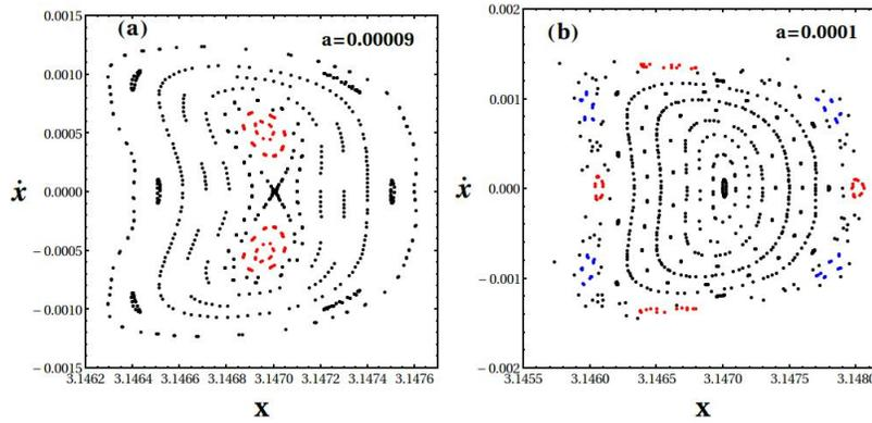
**Figure 4.** A zoom in of the Poincaré surface of section  $(x, \dot{x})$ , for  $y = 0$  and  $\dot{y} > 0$  (a) for  $\alpha = 0.00009$ . The basic period-9 periodic orbit is unstable (black). The red islands of stability correspond to the two stable period-9 periodic orbits bifurcated from the basic one. (b) for  $\alpha = 0.0001$ . The basic period-9 periodic orbit is stable. Two stable period-36 orbits are marked in blue and red around the basic period-9 orbit.
