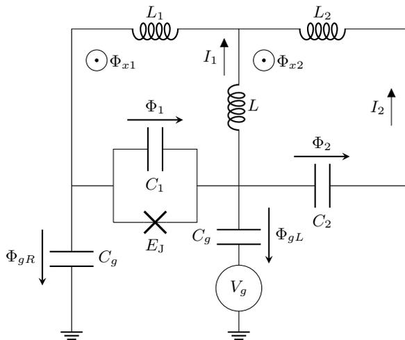
FIG. 2. (a) Equivalent circuit of a two-loop superconducting device. Loop 1 containing a Josephson junction implements the AA, and loop 2 plays the role of the mode. The system is driven by a gate voltage  $V_g(t)$  acting on the AA's charge ( $q$ -port) and possibly biased by external magnetic fluxes  $\Phi_{xi}$  concatenated with each loop  $i = 1, 2$  ( $\gamma$ -port).
