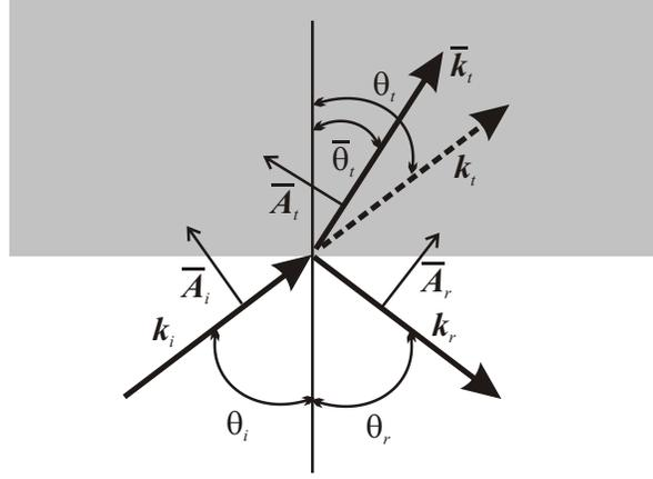
FIG. 2: Convention used for the case of a dielectric with a transverse incident wave whose polarization corresponds to the magnetic field parallel to the interface (normal to the plane of the figure).
