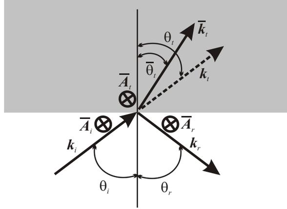
FIG. 3: Convention used for the case of a dielectric with a transverse incident wave whose polarization corresponds to the electric field parallel to the interface (normal to the plane of the figure).
