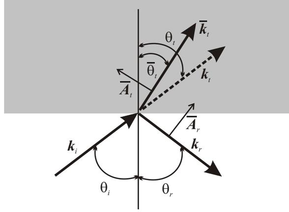
FIG. 1: Sketch of the incident ( $i$ ), reflected ( $r$ ), and transmitted ( $t$ ) waves at the interface between vacuum (below) and material medium (above). The overline denotes the transverse component parameters.
