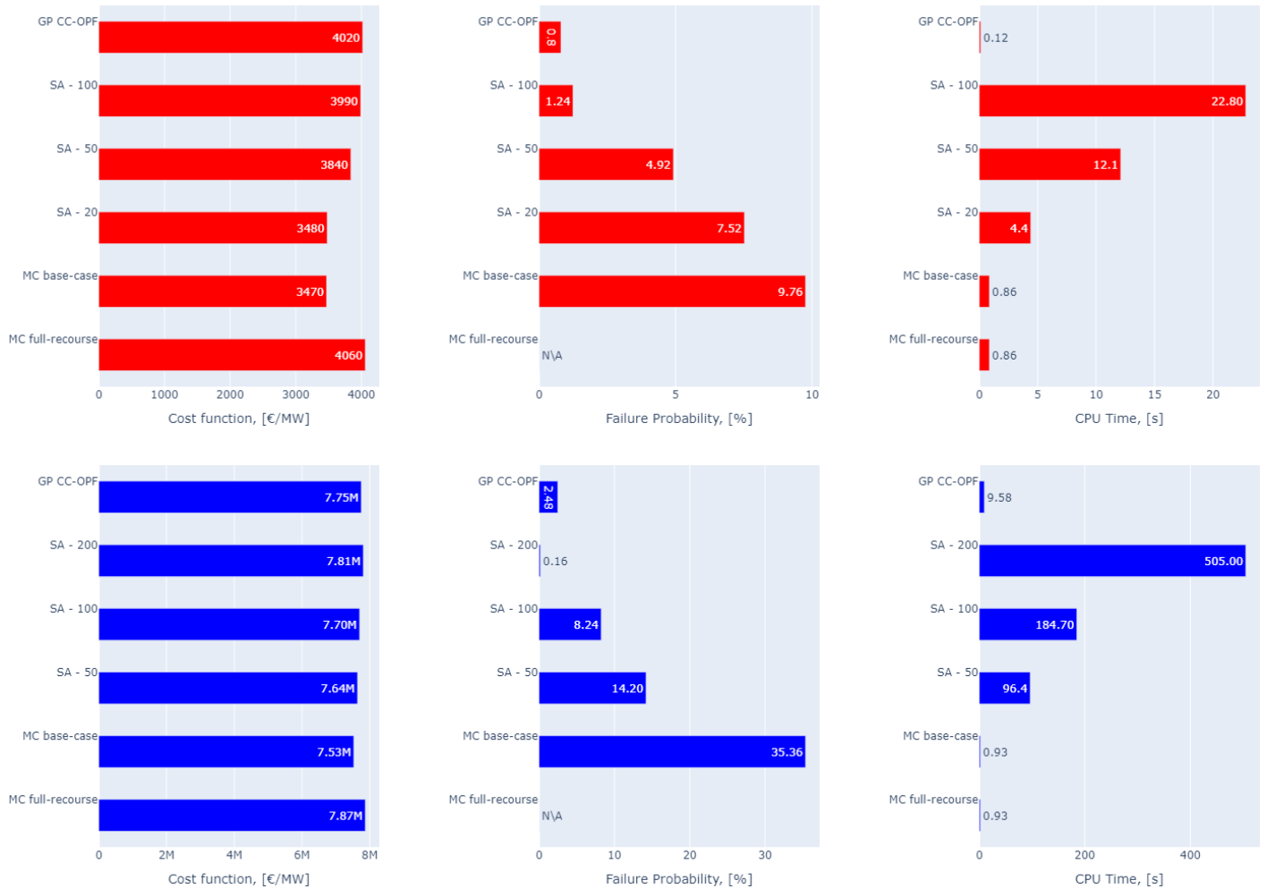
Figure 2: Cost function values, probability of a failure and CPU time for IEEE9 (red) and IEEE39 (blue) systems.
