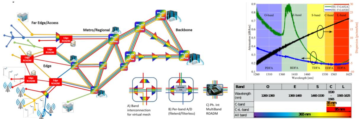
Figure 3: MB network architecture with per-band differentiated reach and services (left); MB switching/ROADMs (bottom); MB considered spectrum with measured loss of G.652D fibre (right)
