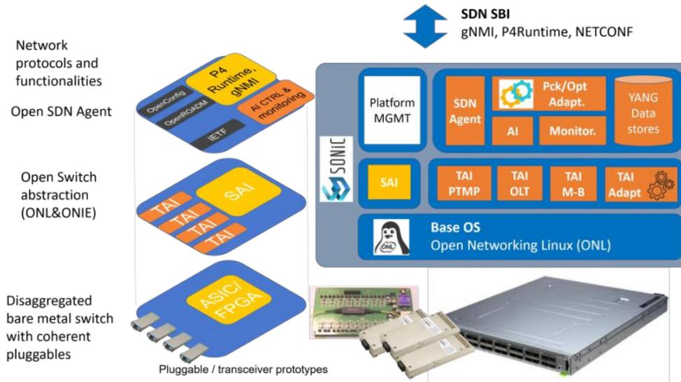
Figure 4: Open packet-opto operating system (in orange the novel SW components).
