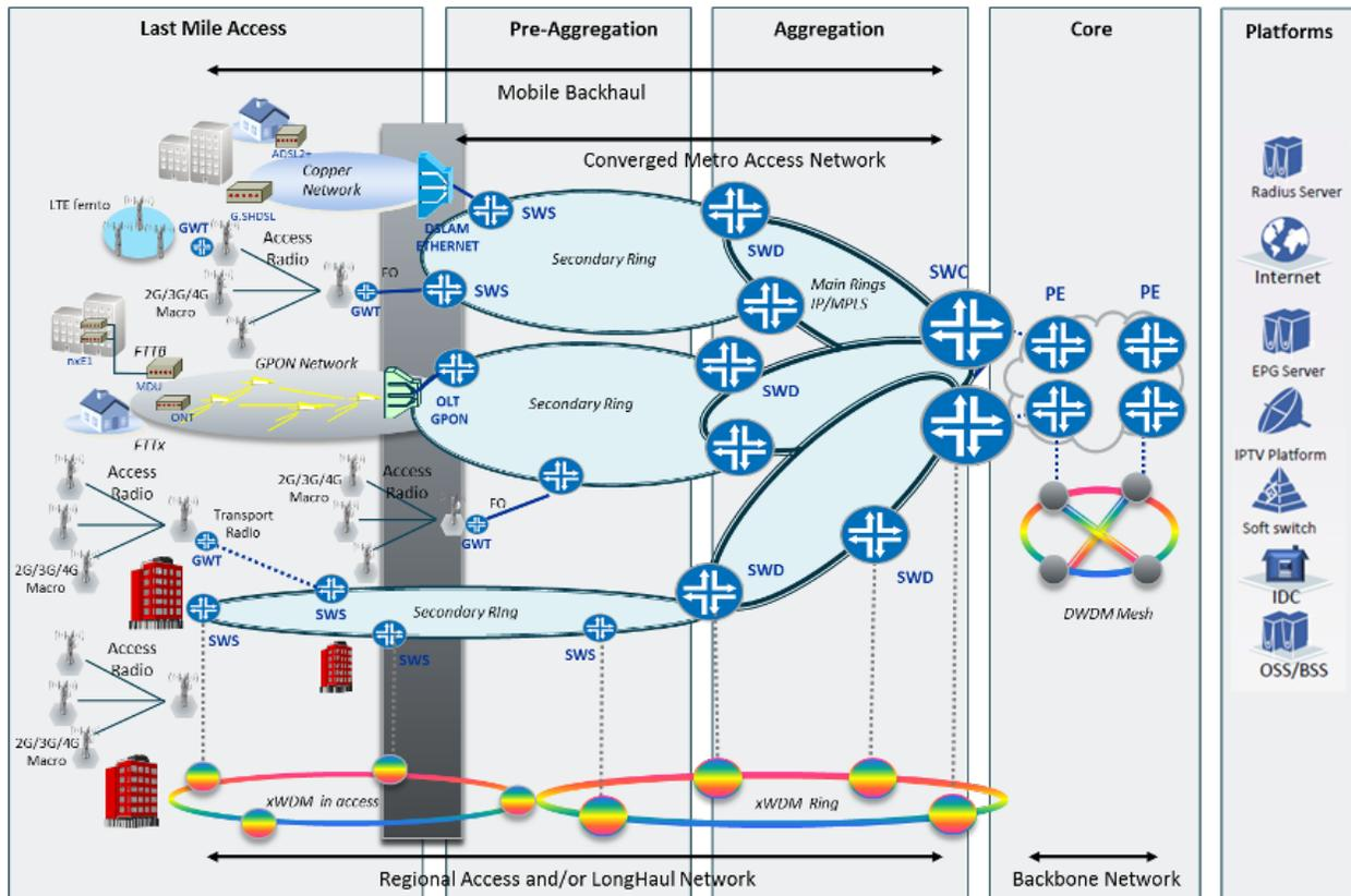
Figure 1: Hierarchical and domain-segment architecture of telco operators
