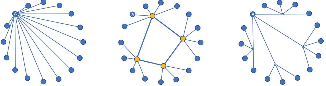
Figure 5: Connectivity solutions based on: direct interconnection in full mesh (left); hierarchical electronic grooming (center); proposed direct interconnection through point-to-multipoint pluggable transceivers over MB in packet-optical nodes.
