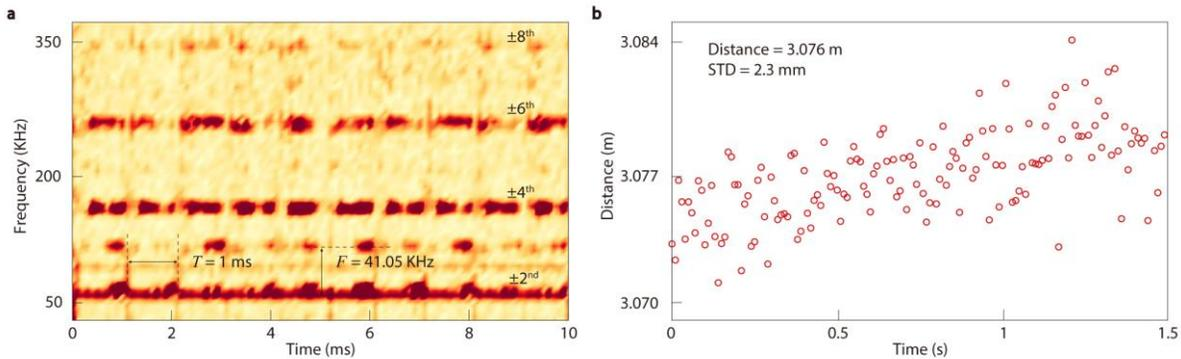
**Fig. 5| Experimental results of the distance measurement by sweeping the repetition rate of OAM-EOFC. a,** Measured spectrum as a function of time. The sweeping period  $T$  of the modulation signal is 1ms. The average frequency difference between adjacent beat frequencies  $F$  is 41.05 KHz. **b,** Measured absolute distances as a function of time.
