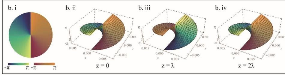
(b) Tracking of angular rotation for a  $LG_{02}$  phase distribution
