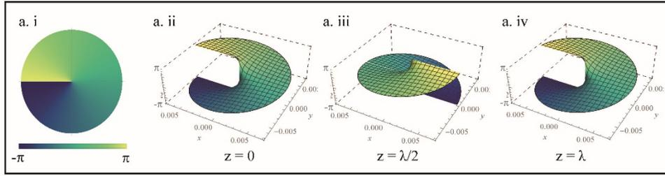
(a) Tracking of angular rotation for a  $LG_{01}$  phase distribution
