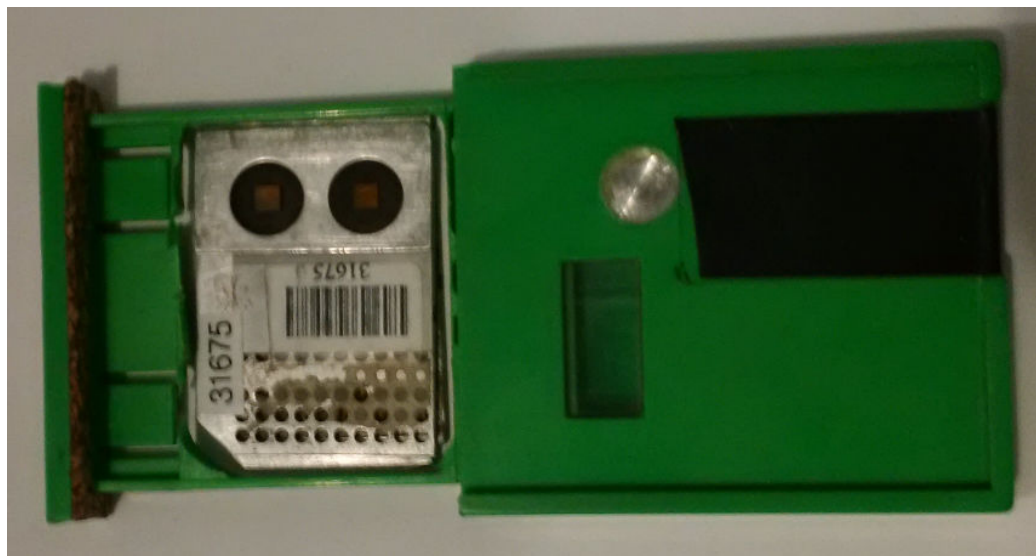
Figure 3. TLD housing (badge) with “thin” (TLD-700) and “thick” (TLD-100) chips were used in this study. To improve statistics, two aluminum plaques with TLD chips were used, one on top of the other. Note that two aluminum plaques, “front” and “rear”, are located in the badge on top of each other.
