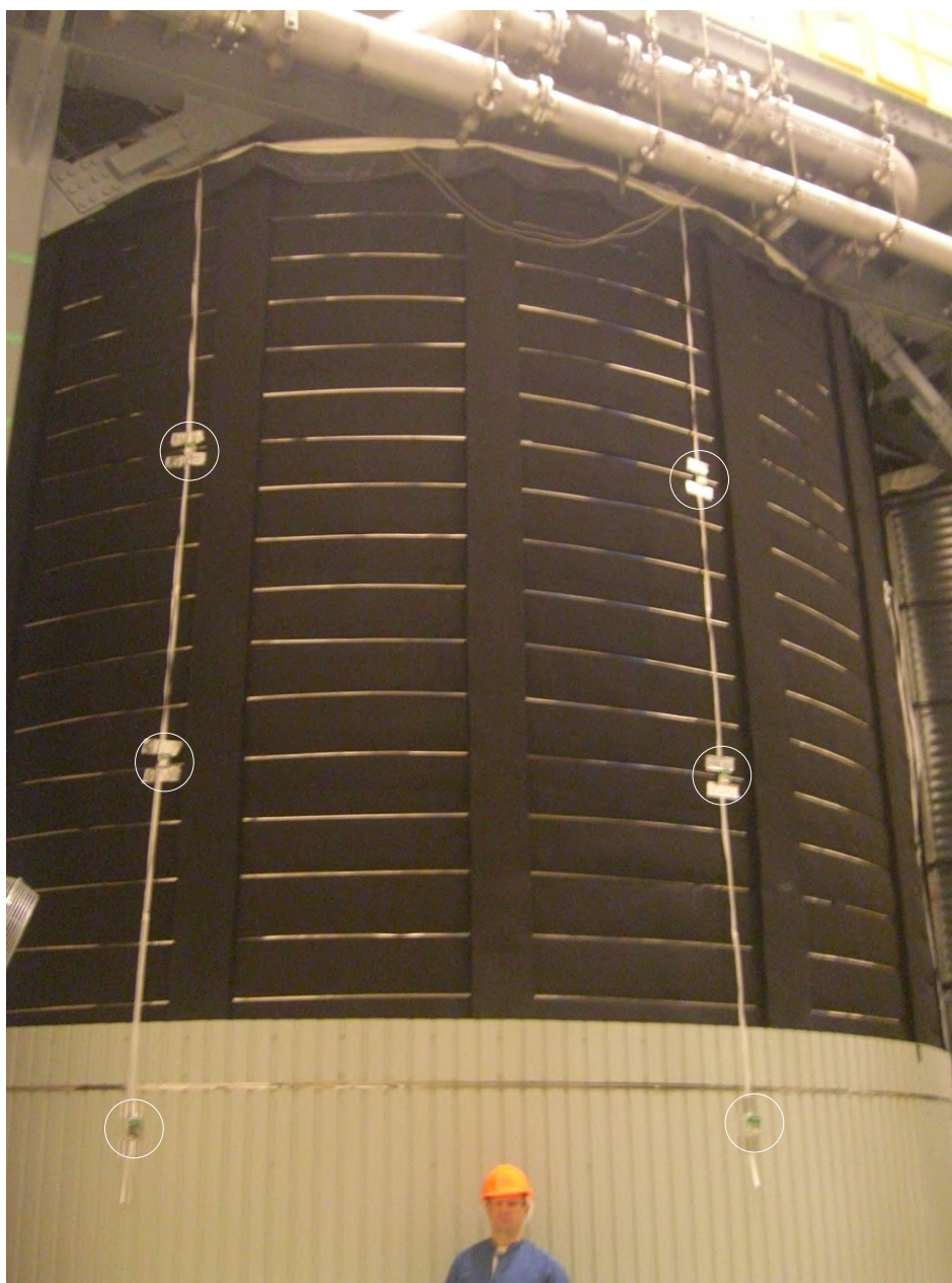
Figure 4. Integrating passive TLD detectors deployed at DEAP-3600 water shielding. Six of the badges, circled in the picture, were distributed around the water shield. Each badge contained two TLD-100 chips (see Figure 3) practically at the same spot. TLDs that were hosted inside badge ID 29 (see Table 1) were placed at the top of the DEAP-3600 water shielding. The MiniCLEAN water tank is also partially shown.
