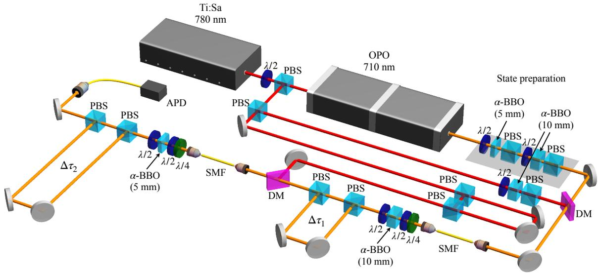
FIG. 3. **Experimental setup.** Experimental setup demonstrating the measurement of ultrafast time-bin qudits in dimension  $d = 4$ . Ti:Sa: Titanium Sapphire laser;  $\lambda/2$ : Half-wave plate;  $\lambda/4$ : Quarter-wave plate; PBS: Polarizing beam splitter; OPO: Optical parametric oscillator; ND: Neutral density filter; BS: beam splitter; DM: Dichroic mirror; SMF: Single mode fibre; APD: Avalanche photodiode detectors.
