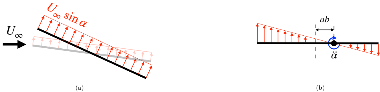
FIG. 3. Illustration of added-mass components i (a) and ii (b) in eq 2 for a pitching-up wing
